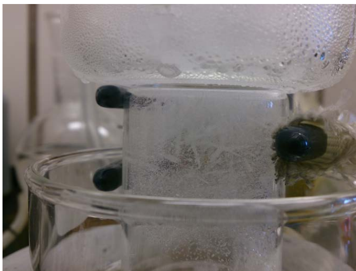
Figure 7. Formation of Pure 3,5-bis(trifluoromethyl)pyrazole crystals via sublimation.
