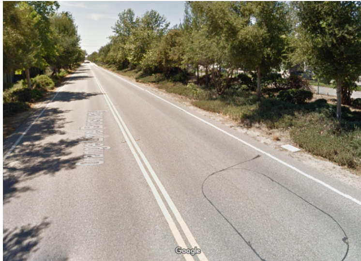
Figure 4. An upstream loop detector (bottom right) (Google, 2014).
