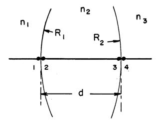
Fig. 4. Thick lens.
