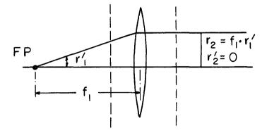
Fig. 7. Definition of the FL for a thin lens.
