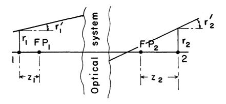
Fig. 9. Definition of z<sub>1</sub> and z<sub>2</sub> for Eq. (15) (z<sub>1</sub> and z<sub>2</sub> are positive in this figure).
