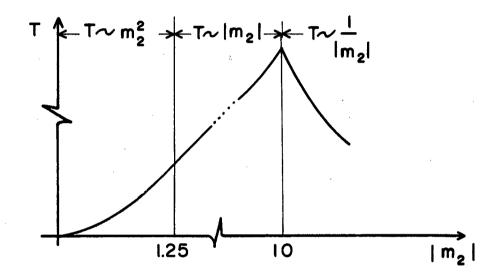
Fig. 22. Light transmission, T, as a function of  $|m_2|$  for a spectrometer setup.
