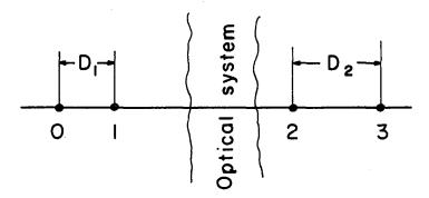
Fig. 6. Relative position of RP's for the derivation of Eq. (9) (D<sub>1</sub> and D<sub>2</sub> are positive in this figure).
