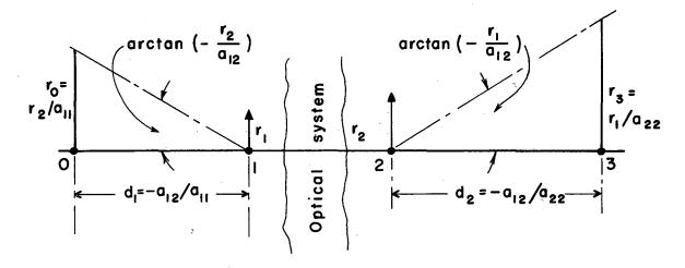
Fig. 18. Projection of RP's (or apertures) for  $\frac{n_1/n_2}{\log n_1} = 1$  (d<sub>1</sub> and d<sub>2</sub> are positive in this figure).
