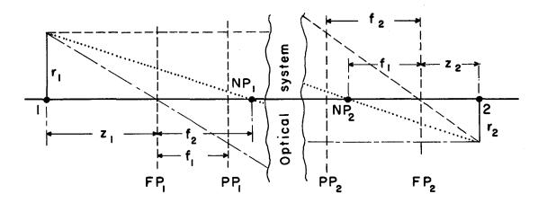
Fig. 10. Geometrical image construction and relative positions of FP's, PP's, and NP's of an optical system with positive FL's.
