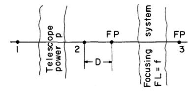
Fig. 15. Combination of a telescope and a focusing system.
