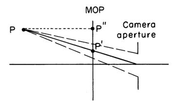
Fig. 19. Limitations of resolution because of parallax and the size of the camera aperture.
