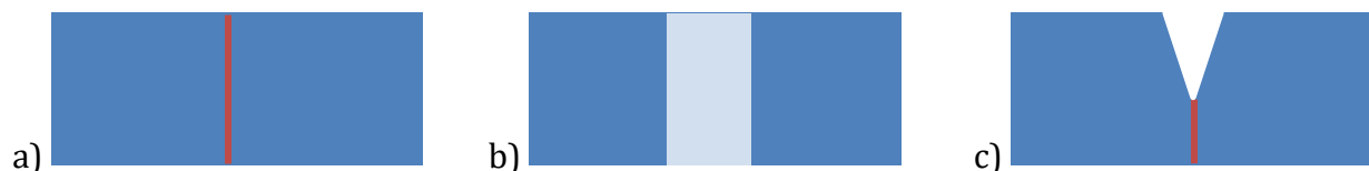
Figure 1.2 Cartoon of the etch process for both cylindrical and conical pores. (a) A damage track is made through a membrane. (b-c) Etching processes for a cylindrical pore and conical pore. In the cylindrical pore fabrication (b) , the damage track etches through very rapidly by comparison to the bulk, allowing an even etching of the entire pore, which gradually widens. In the conical pore case (c) , the track etch rate is slowed to the point where the bulk etching of the inner membrane can occur at a more comparable pace, which results in the conical shape over time.
