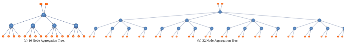
Figure 4.15: Aggregation Tree based sNoC topology.
