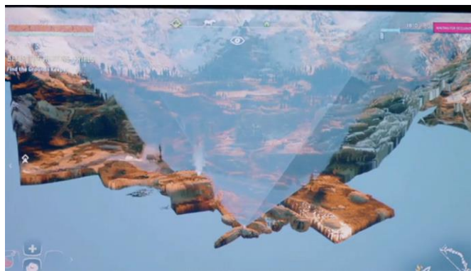
Figure 15: Frustum culling, evidenced by the blue area in the lower half of the image, removes graphical elements “behind” a player-character and out of their visual range.
