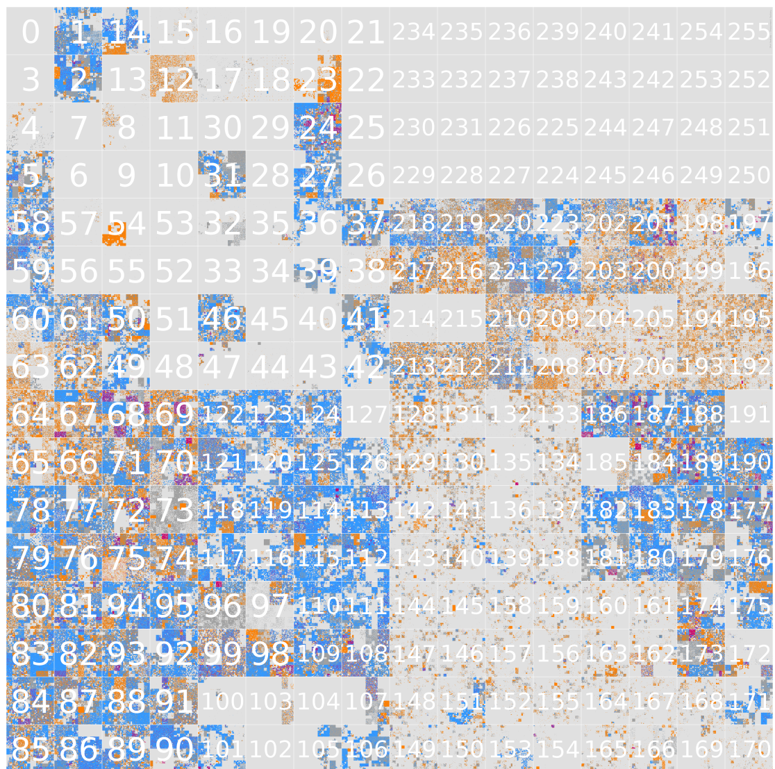
Figure 6.4. Hilbert curve of the IPv4 address space showing host functionality. Light grey indicates unused, dark grey used unclassified, blue client, orange server, pink routing infrastructure.
