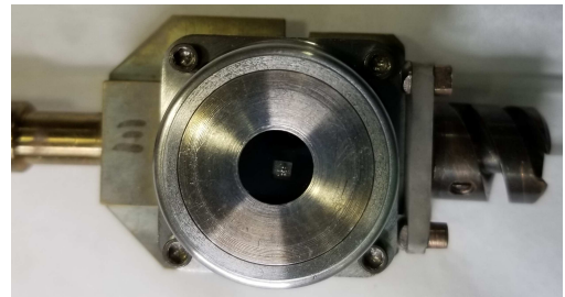
Figure 3.4: A 1cm x 1cm Si Frame with a 2cm x 2cm SiN membrane mounted in a PEEM-3 sample holder. Sample S30 from section 4.3.3 is visible.
