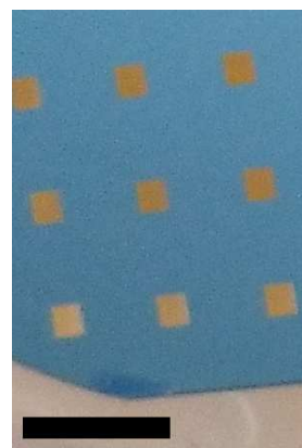
Figure 3.1: An optical image of a Si wafer with an array of 2mm x 2mm a-SiN x membranes. Scale bar is 1cm.
