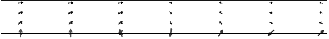
Figure 2.5: OOMMF simulation showing a cross sectional cut of a 30nm thick 1 \mu m diameter Permalloy disk on top of 10nm of [Pt/Co/Ir] multilayers. The disk is canted out of plane by the multilayers below.
