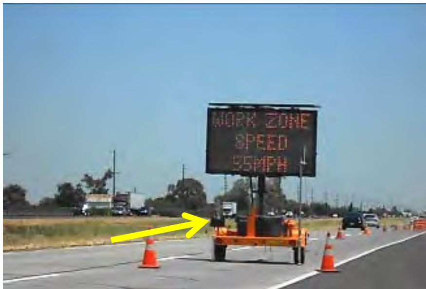
Figure 16. Location of Radar Sensor on CMS Trailer
