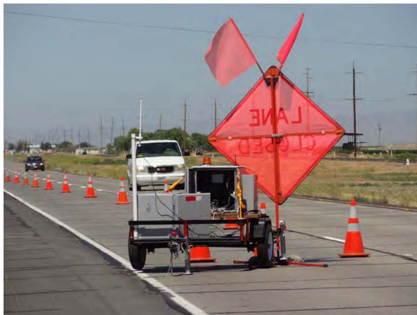
Figure 7. Placement of Speed Camera
