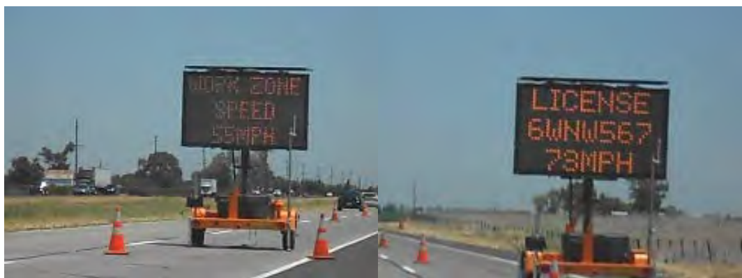
Figure 3. Display on Changeable Message Signs in Field Tests
