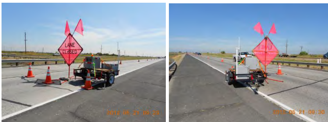
Figure 2. Placement of Speed Camera Trailer in Field Tests; At left, photo taken in traffic direction in front of the speed camera; At right, facing traffic behind the speed camera.
