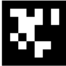
Figure 2.3: AprilTag 2D bar code style "tags" to enable 6-DOF localization of features from a single image.
