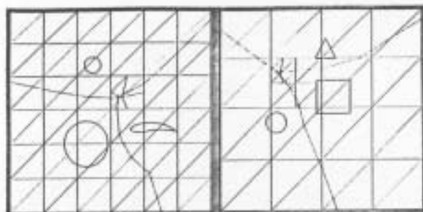
Figure 7 Recursive subdivision of parameter space triangulations for generation of points on bisectors in Voronoi diagram
