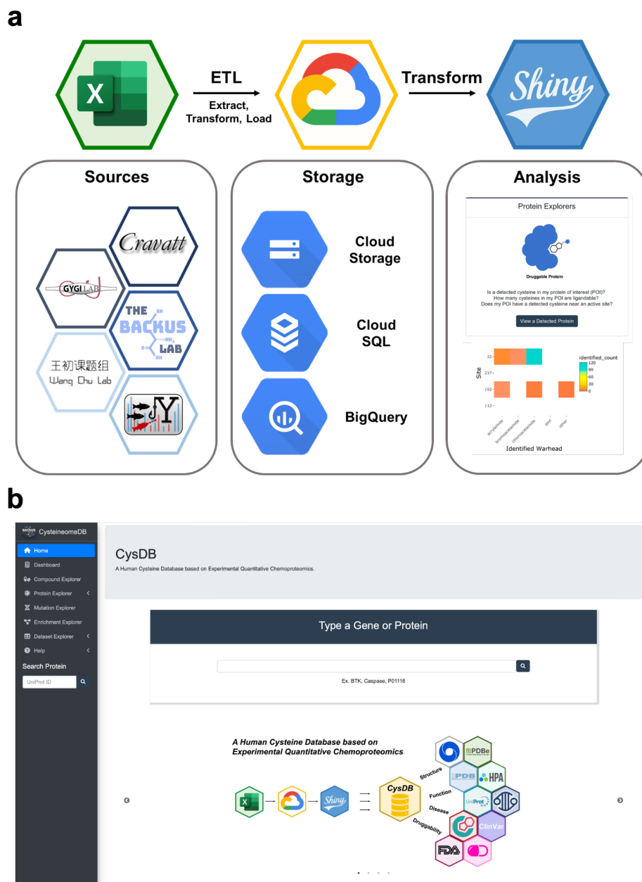
Figure 2. Workflow to generate CysDB SQL database. (A) Data extracted from nine datasets ( Data S1 ) was transformed and loaded into a MySQL relational database on the Google Cloud Platform. An accompanying front-end web interface was developed using RShiny to allow remote-user querying of the SQL database. (B) Homepage of the CysDB app publicly available at https://backuslab.shinyapps.io/cysdb/ . See Figure S6 and Data S1 and S2 .
