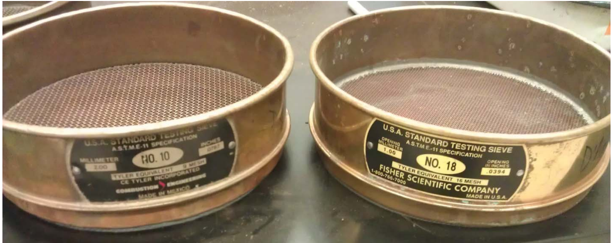
Figure 2: Two sieve sizes were used in order to more efficiently strain out the Nipomo seed. Sieve #10 and #18
