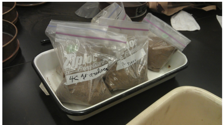
Figure 1: Soil samples were collected and stored in plastic Ziploc and left open in order to dry.
