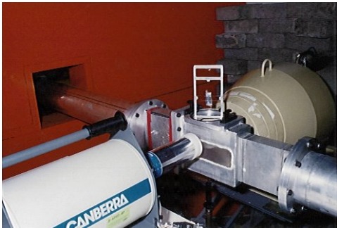
Figure 1. The Budapest Reactor cold neutron beam experimental facility. A 25% HPGe detector (foreground) is shown pulled away from its Compton suppression system (background). The target assembly is shown in its external position. The 5 \times 10^7 n/cm 2 s neutron beam arrives from the right in the neutron guide. We propose replacing the current detector with 2 clover detectors that can achieve high coincidence efficiency in a close geometry and do not require Compton suppression because of their photon add-back capability.
