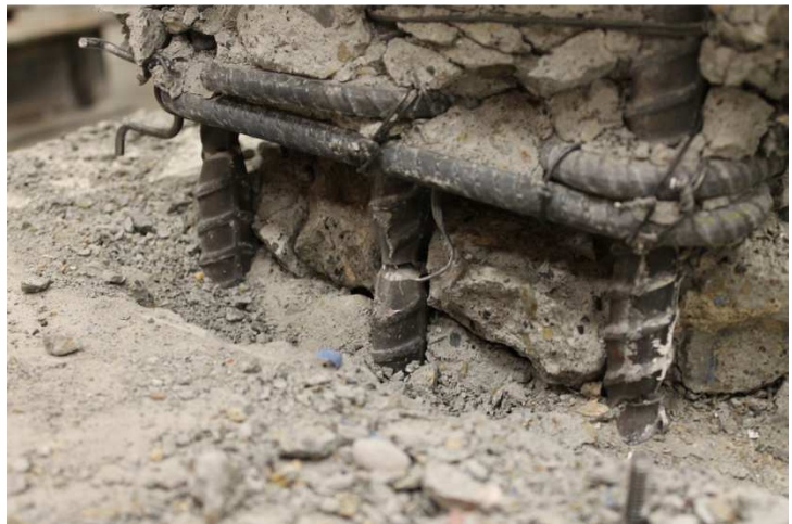
Figure 4.3.4: Failure Mechanism of SBM100 by Fracture of Longitudinal Bars
