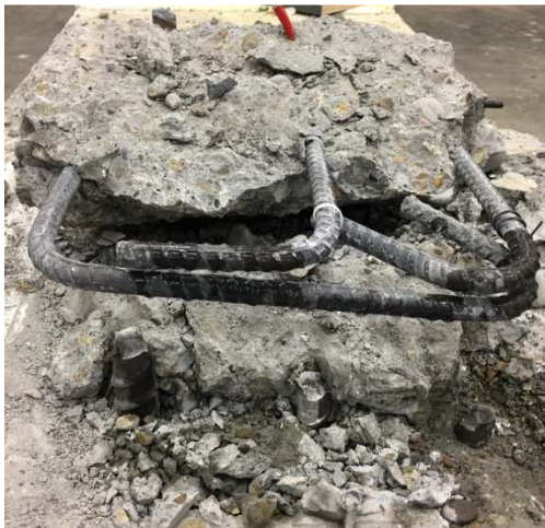
Figure 4.3.4: Failure Mechanism of SBM100 by Fracture of Longitudinal Bars
