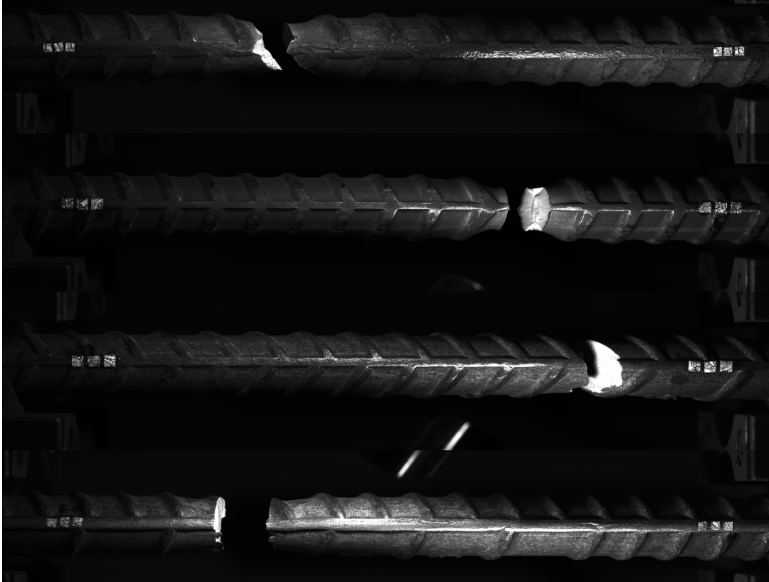
Figure A-16: Typical Photograph from DIC System in Bar Tests – From Top Down: A706 Gr. 60, Gr. 100 A1035, Gr. 100 with T/Y = 1.17, and Gr. 100 with T/Y = 1.26.
