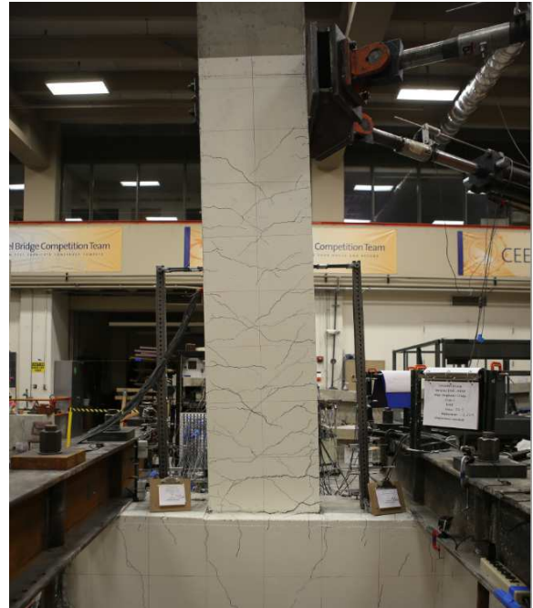
Figure 4.1.3: Deflected shape of SBL100 at Drift Ratio 2.45% (Left) and 3.45% (Right).
