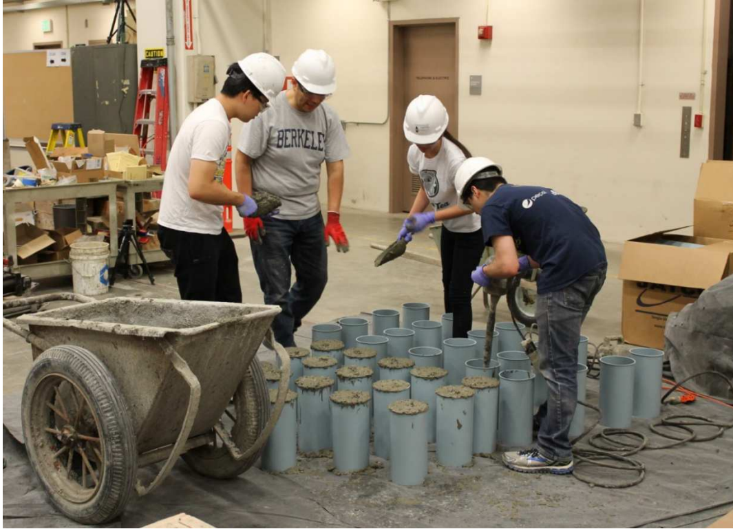
Figure A-6: Casting Concrete Cylinders
