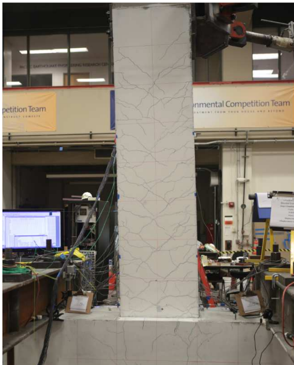
Figure 4.1.4: Deflected shape of SBM100 at Drift Ratio 2.45% (Left) and 3.45% (Right).
