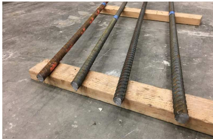
Figure A-15: Longitudinal Steel Used in Test Specimens - Left to Right: SBL100, SBH100, SBM100, SBH60
