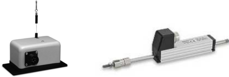
Figure A-24: Typical Displacement Transducers Used in Tests. Left: String Potentiometer for Global Deflection Measurement; Right: Novotechnik Used to Measure Local Deformations
