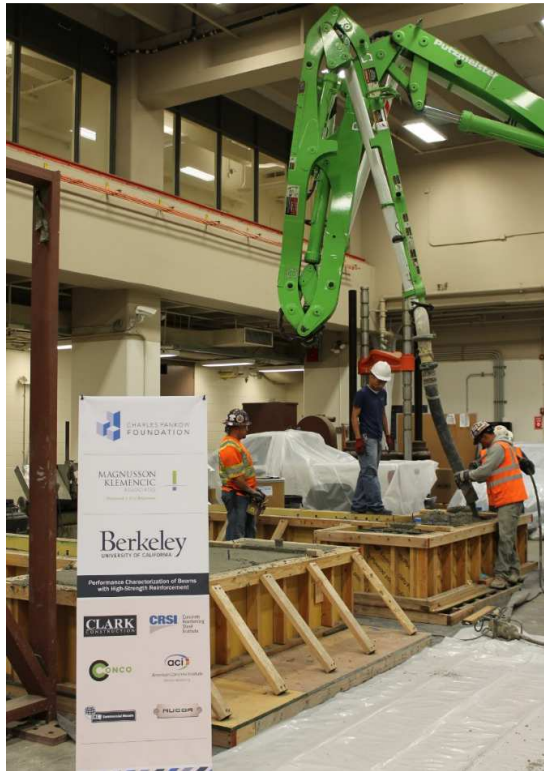
Figure A-5: Construction of Test Specimens - Concrete Casting
