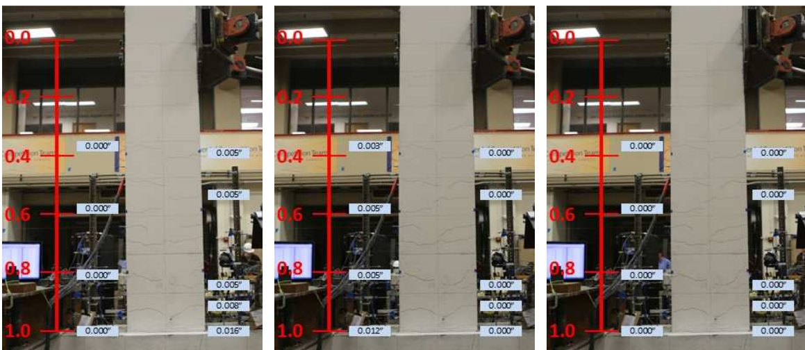
Figure C-2: Measured Crack Widths at Drift Ratio of 0.5% – Specimen SBH60
