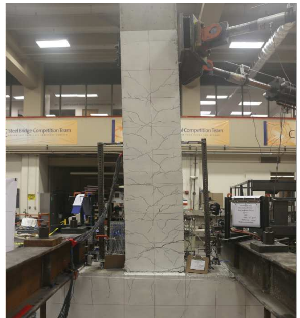
Figure 4.1.2: Deflected shape of SBH100 at Drift Ratio 2.45% (Left) and 3.45% (Right).
