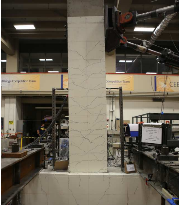
Figure 4.1.3: Deflected shape of SBL100 at Drift Ratio 2.45% (Left) and 3.45% (Right).
