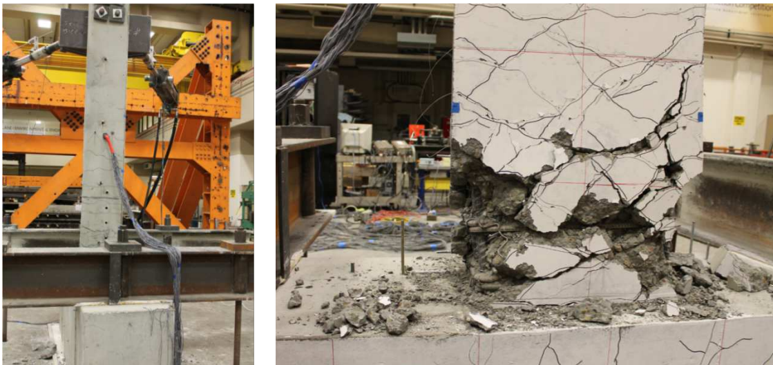
Figure 4.3.1: Failure Mechanism of SBH60 by Twisting of Beam (Global Instability)
