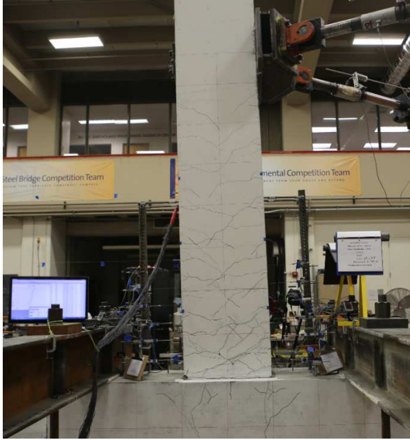
Figure 4.1.1: Deflected Shape of SBH60 at Drift Ratio 2.45% (Left) and 3.45% (Right)
