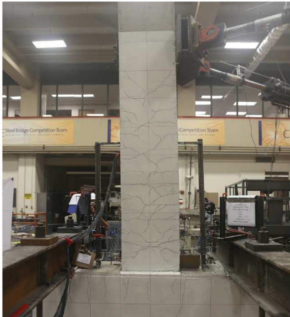
Figure 4.1.2: Deflected shape of SBH100 at Drift Ratio 2.45% (Left) and 3.45% (Right).
