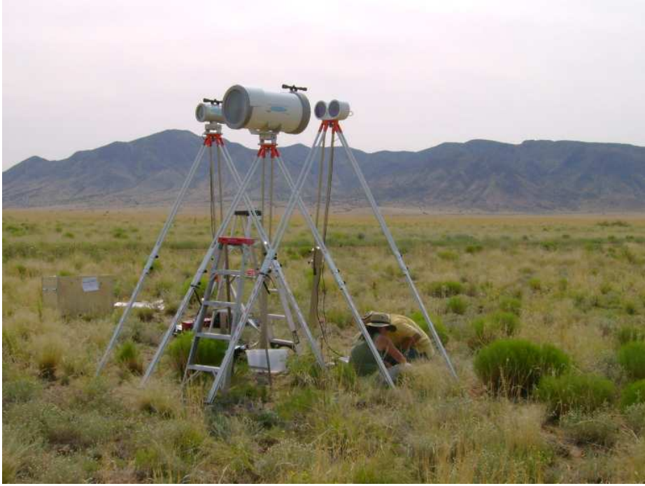
Fig. 2 Photograph of the south-east set-up with (from left to right) LASL1050m transmitter, XLAS receiver, BLS900 transmitter. The receiver of LASL544m is 10 m to the right.
