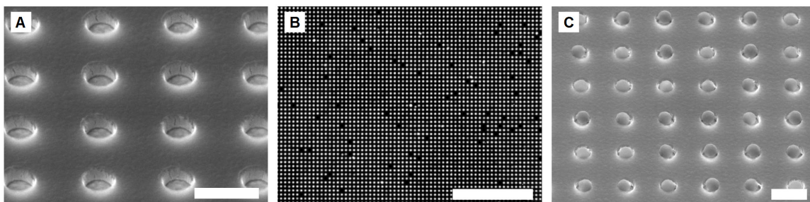
Figure 3-4. Arrays of microwells and antibody-conjugated microbeads. (A) SEM image of a small portion of an array of \sim 0.5 \mu\text{m} wells at a 1.2 \mu\text{m} pitch etched in a silicon dioxide film that was deposited on a gold-coated wafer. (B) Raw fluorescence image of a small portion of an assembled array of 0.4 \mu\text{m} antibody-conjugated beads at a 1.2 \mu\text{m} pitch. (C) SEM image of a small portion of an assembled array of 0.4 \mu\text{m} antibody-conjugated beads at a 1.2 \mu\text{m} pitch. The scale bars in (A) and (C) are 1 \mu\text{m} . The scale bar in (B) is 24 \mu\text{m} .
