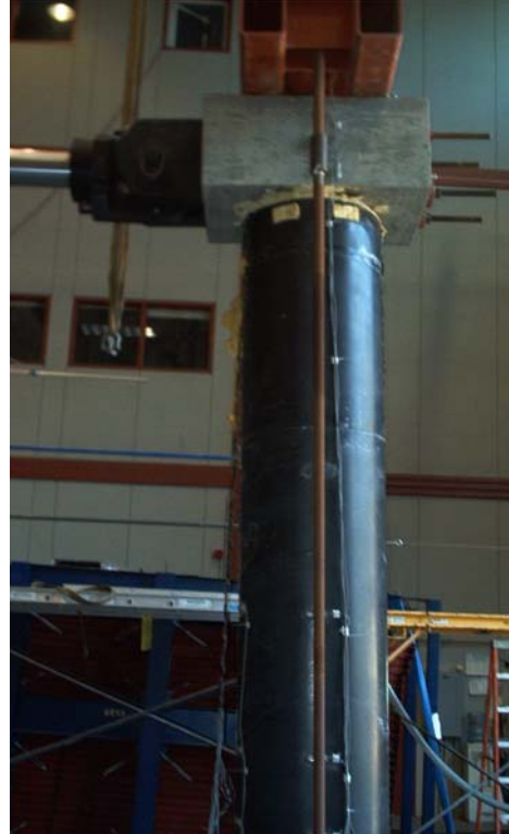
Figure 4-7: Overview of Flexure Test Set-Up
