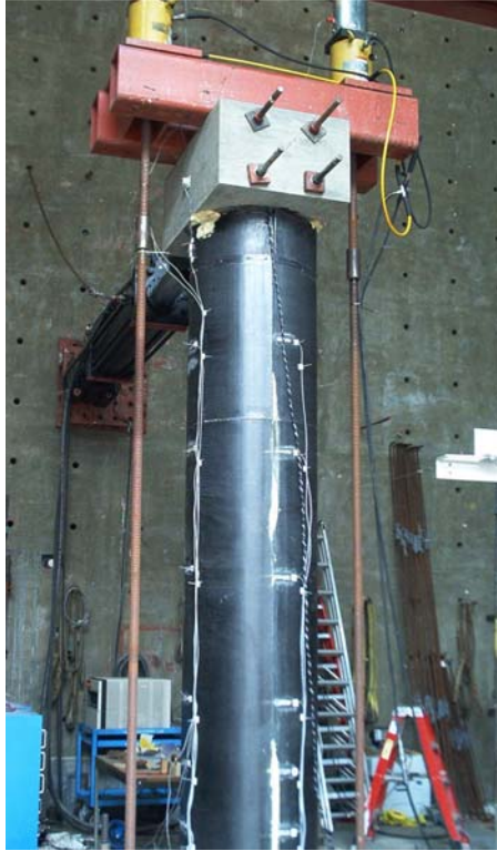
Figure 4-6: Overview of Flexure Test Set-Up
