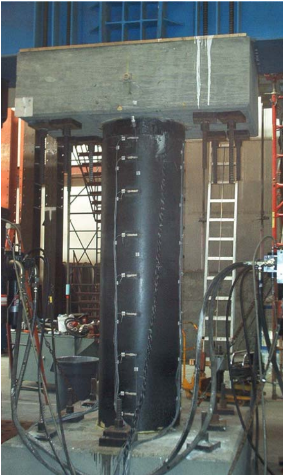
Figure 3-27: Shear Column during Load Controlled Cycling
