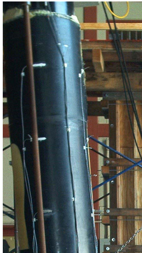
Figure 5-19: Lapped Reinforced Circular Flexural Column during testing
