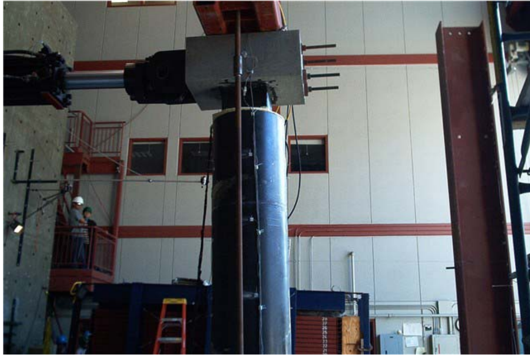
Figure 5-47: Lapped Reinforced Square Flexural Column during testing
