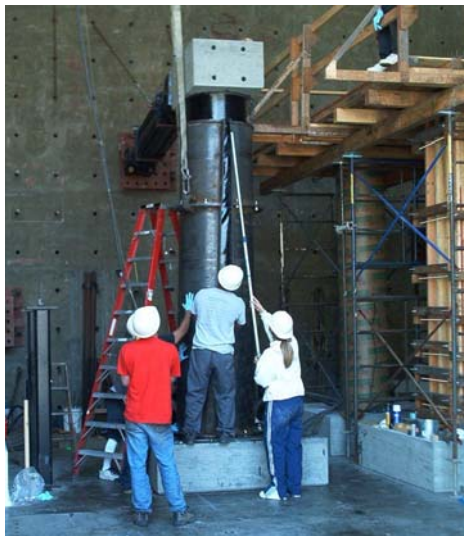
Figure 2-26: Lapping of the Jacket Seams Figure 2-27: Pouring of Expandable Foam Core
