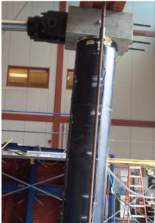
Figure 4-20: Continuously Reinforced Circular Flexural Column during testing
