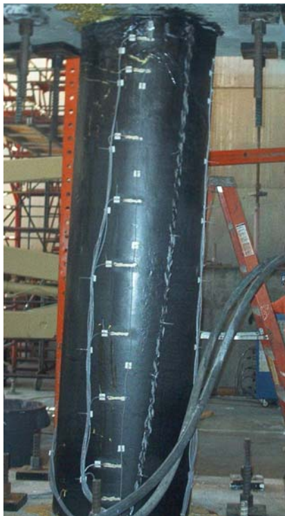
Figure 3-52: Shear Column during testing
