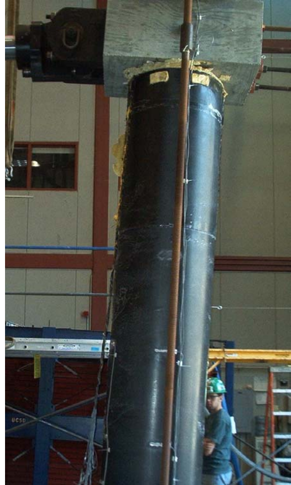
Figure 4-44: Continuously Reinforced Square Flexural Column during testing
