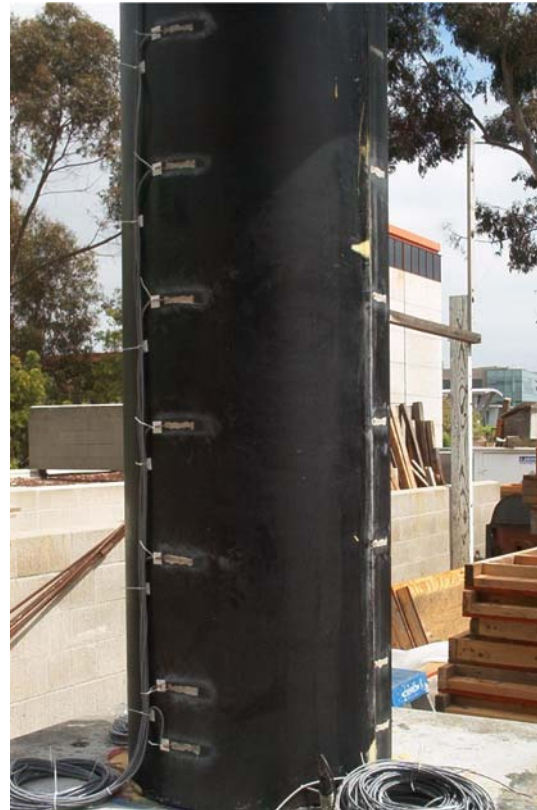
Figure 3-12: Jacket Strain Gages at North and West Faces of Shear Column
