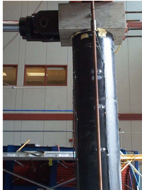
Figure 4-21: Continuously Reinforced Circular Flexural Column during testing
