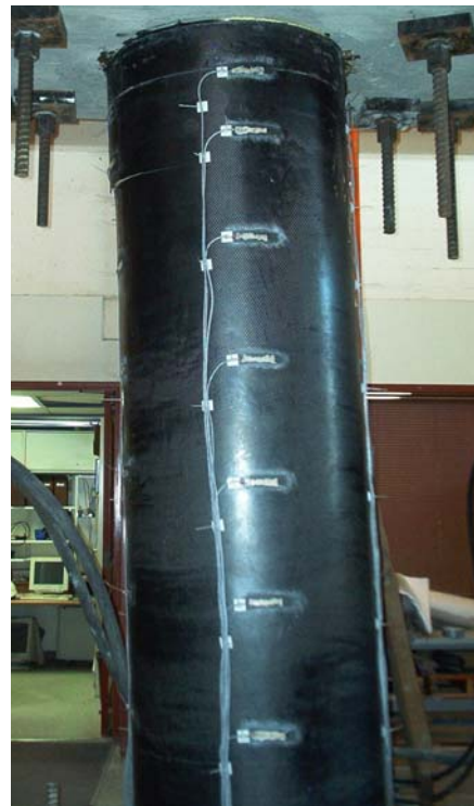
Figure 3-53: Column under 9.7 cm Deflection
