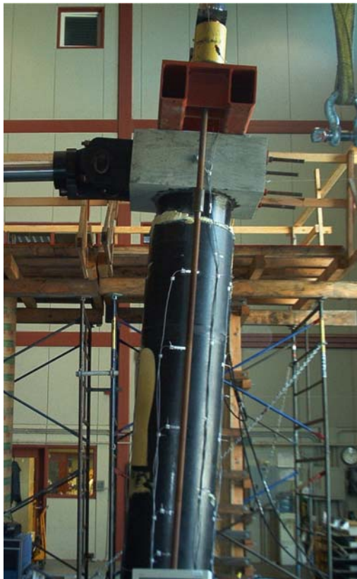
Figure 5-18: Lapped Reinforced Circular Flexural Column during testing
