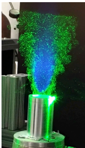
Figure 13. Image of laser sheet (green) through seeded flame (blue)
