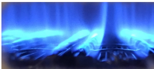
Figure 3. Image of Rheem ECOH200DVLN burner as viewed through the site-glass. The small, bright-blue flames are the fuel-rich regime and the pale-blue, almost transparent flames are the fuel-lean (oxygen-rich) regime.
