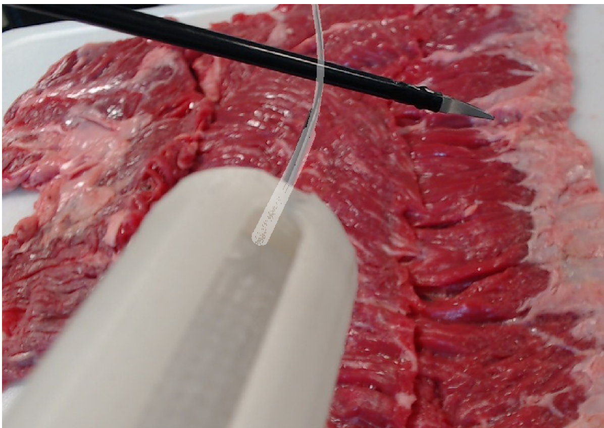
Figure 5.1. An example of robust image segmentation for a concentric tube continuum robot. The robot is successfully identified, as illustrated by the white overlay, despite the presence of multiple, partial occlusions and a background of similar color.
