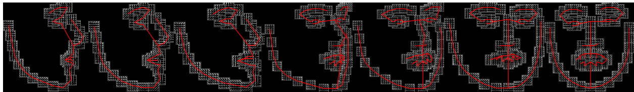
Figure 5.2: Our mixture-of-trees model encodes topological changes due to viewpoint. Red lines denote springs between pairs of parts; note there are no closed loops, maintaining the tree property. All trees make use of a common, shared pool of part templates, which makes learning and inference efficient.
