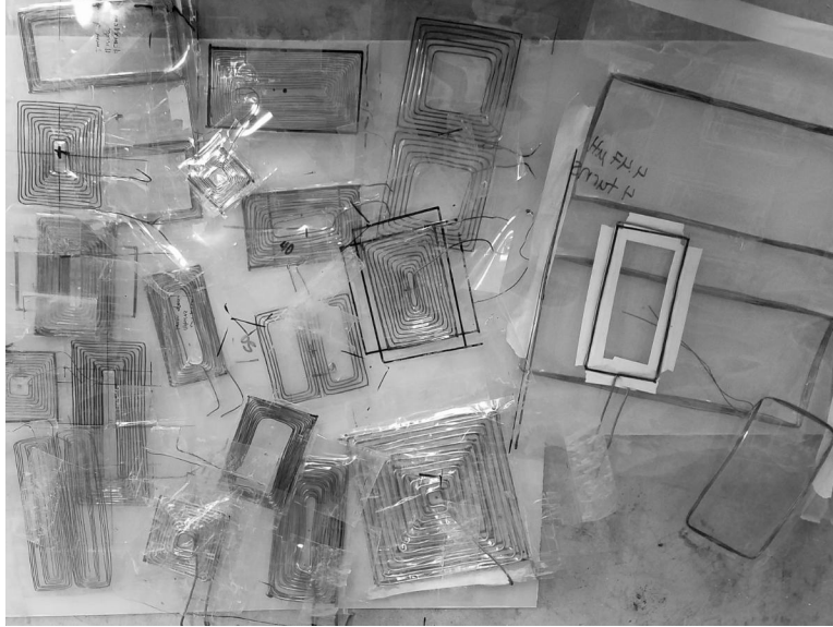
Figure 3.1. Designing coils by trial and error is a time-consuming and laborious process. This shows a sample of the numerous iterations that were built and tested on the path of designing a coil for one system.
