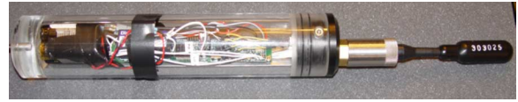
Fig. 1. Autonomous instrument package for recording acoustics, pressure, temperature, and inclination data to a 1-GB flash memory chip. The device can be powered by 4-AA batteries (shown here), although 4 AAA were found to be sufficient.
