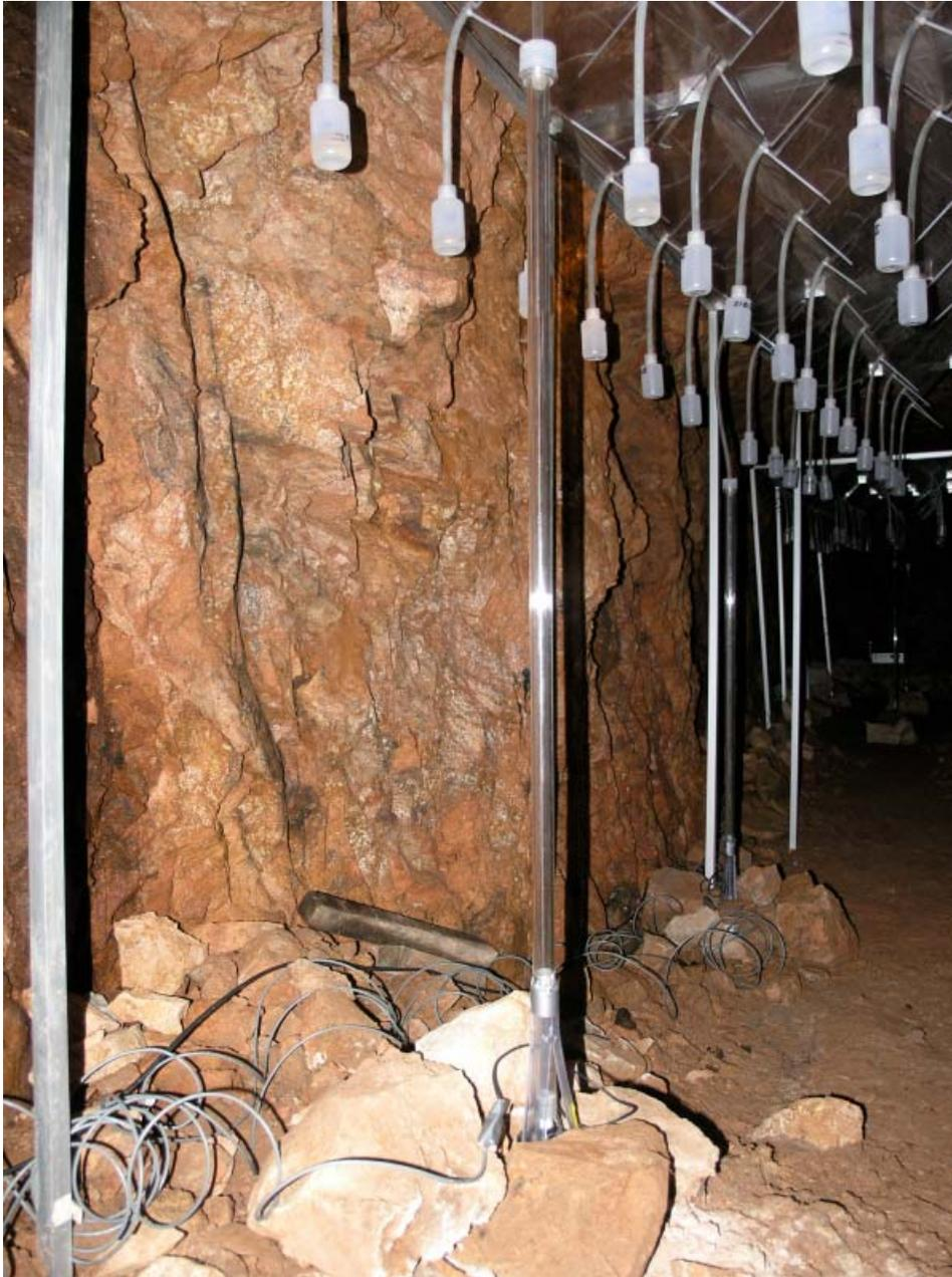
Fig. 3 Array of collection bins and instrumented collection columns (sites 24C, 18A, 8C, and 3C, from foreground to background) within adit seepage collection system
