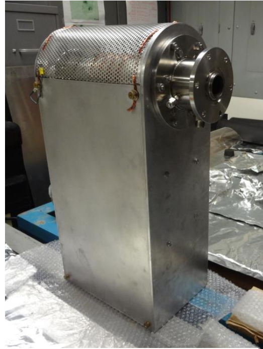
Fig. 23 – Plasma torch and capacitor bank box vertically positioned.
