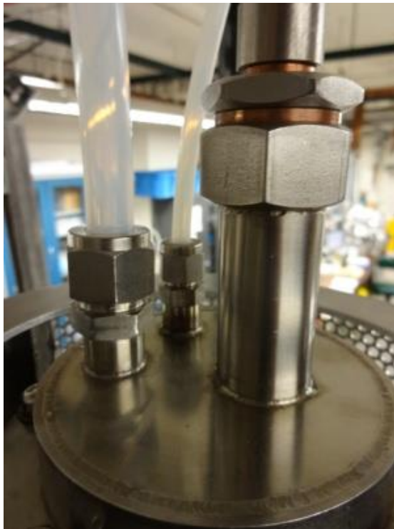
Fig. 7 – Top of plasma torch. (From left to right: \frac{1}{2} " Swagelok outlet for cooling water, \frac{1}{4} " Swagelok fitting for direct vortex plasma gas inlet, ignition rod fitting the top of which has a \frac{1}{4} " Swagelok fitting for compressed gas)
