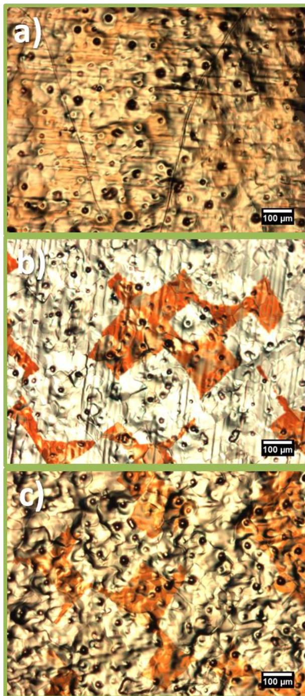
Figure 3.6: Effect of Cu annealing on graphene growth.(a) 150 sccm H 2 under vacuum pressure @ 1020 °C for 1 hr. (b) 500 sccm H 2 at 17 psia at 1020 °C for 1 hr. (c) 500 sccm H 2 at 17 psia at 1020 °C for 5 hrs.
