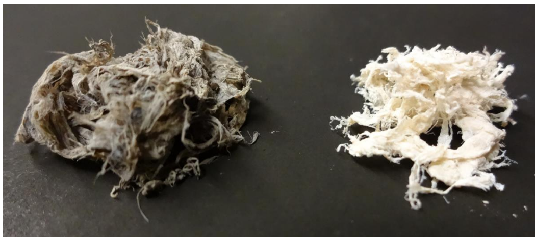
Figure 5.5: Picture of as-synthesized and nitric acid treated material. Chemically treated material (right) can be made much whiter than material collected following a run (left) due to the removal of impurities such as boron.
