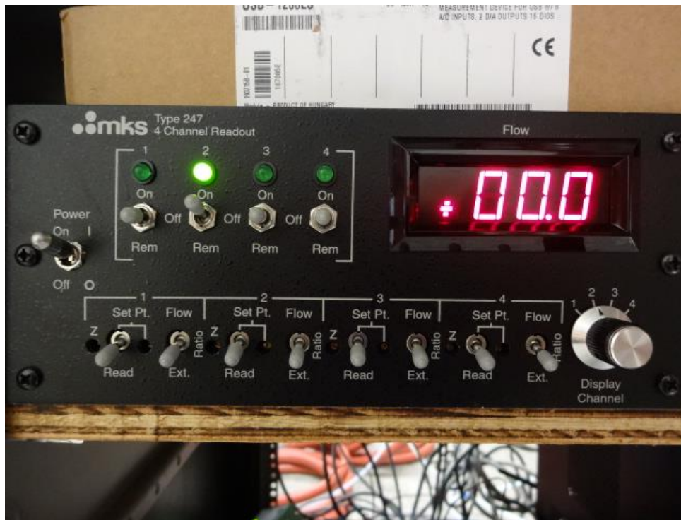
Fig. 14 – MKS Type 247 controller box. (Here the controller box has been switched on, the power to MFC #2 has been switched on, and the display is reading the real flow from MFC #2)
