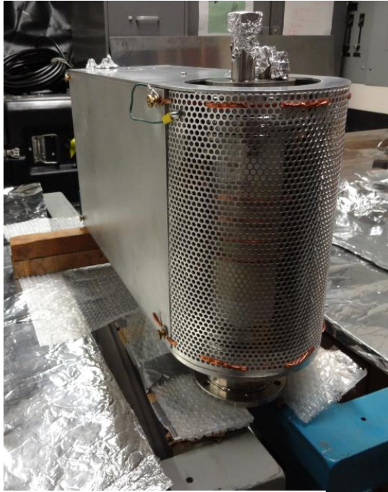
Fig. 22 – Plasma torch and capacitor bank box horizontally mounted in between two tables.
