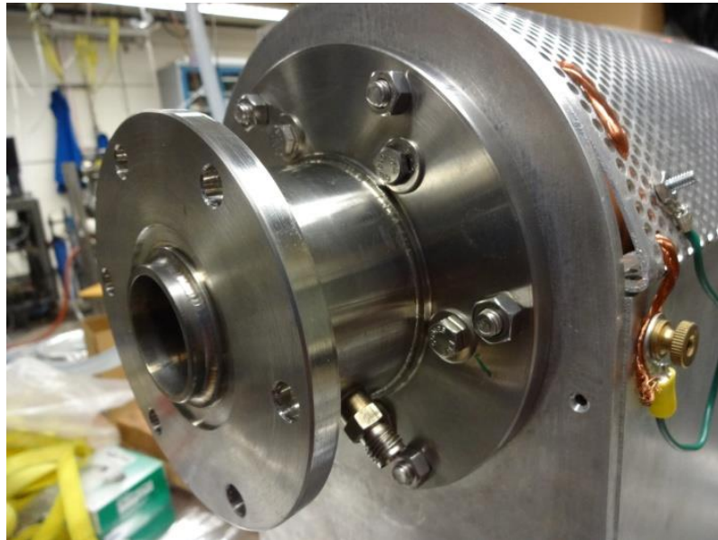
Fig. 25 – Bottom portion of plasma torch (a.k.a. powder feeding chamber).
