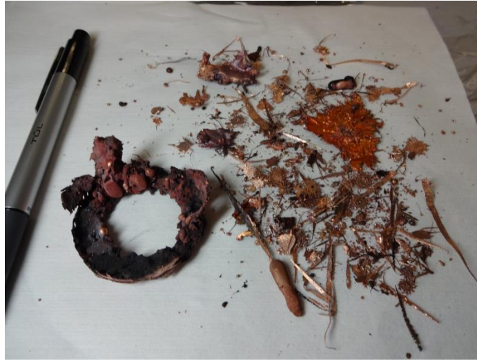
Figure E. 4: Copper pieces collected from inside the synthesis chamber and near the plasma torch exit nozzle.
