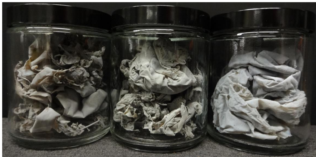
Figure 4.20: Photo of as-synthesized material produced using N_2/H_2 plasma gas mixtures. 50 lpm N_2 gas is mixed with (left) 0% H_2 , (center) 2% H_2 , and (right) 4% H_2 .
