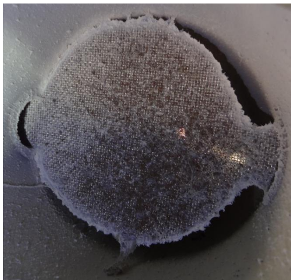
Figure 4.26: Copper mesh collector plate placed downstream plasma torch inside synthesis chamber.
