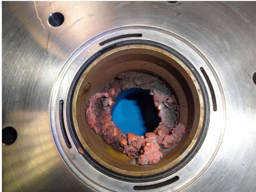
Figure E. 5: Copper collected in powder feeding chamber. Powder feeding chamber is detached from the plasma torch body and is pictured looking down.
