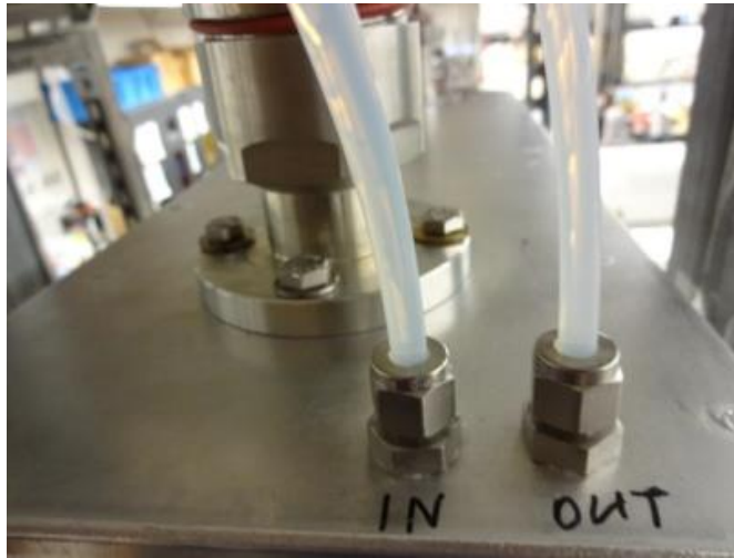
Fig. 8 – Top of capacitor bank box. (From left to right: ¼" Swagelok inlet for cooling water going into capacitor box, ¼" Swagelok outlet for cooling water exiting the capacitor box).
