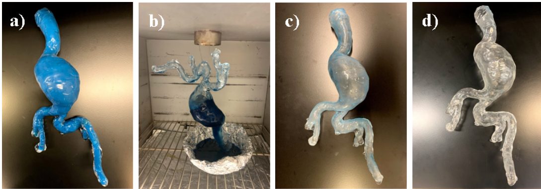
Figure 2.10: Silicone model (a) Silicone coated over the solid wax replica of the abdominal aortic aneurysm model (b) Wax melted out (c) Model after melting out wax (d) Cleaned silicone phantom
