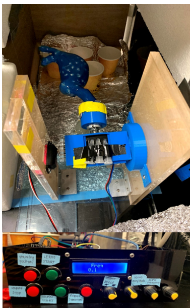
Figure 2.8: Two-axis rotation coating device during the silicone phantom manufacturing process
