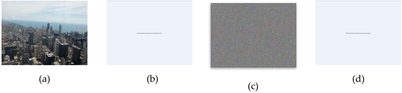
Figure 3.9. (a) the original image; (b) a scrambled image based on the proposed method; (c) a cipher image based on JPEG encoder; (d) cipher image based on AES encryption
