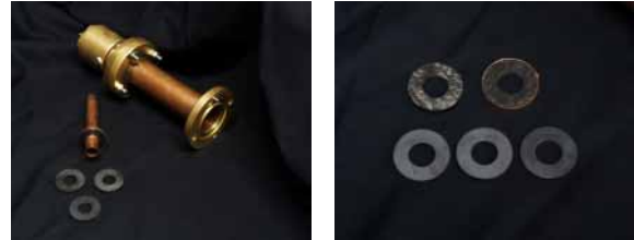
Figure 5. The coaxial air-line test stand used for testing the material samples is shown on the left. The pipe is a 50 \Omega line, has type-N connectors on each end, and has a removable center conductor. The torque of each bolt was set to 50 oz.-in. and was required for calibration purposes.
