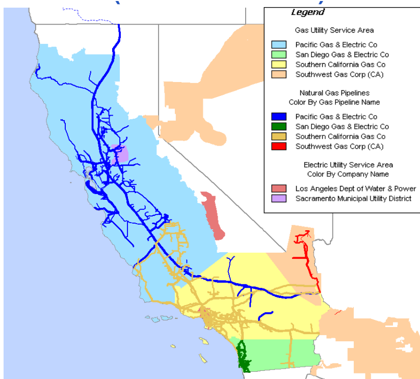
Figure 2-8: Utilities Serving California, Source: Energy Velocity
