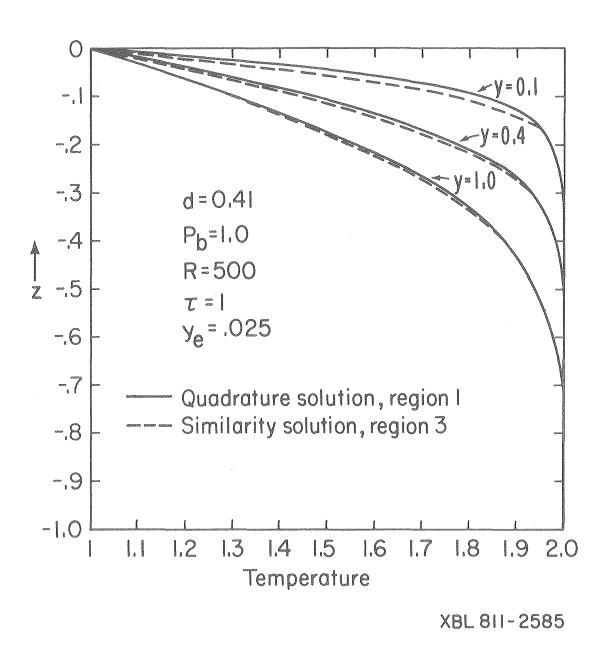
Fig. 8. Fluid temperatures in the near fault regions 1 and 3 of the aquifer.
