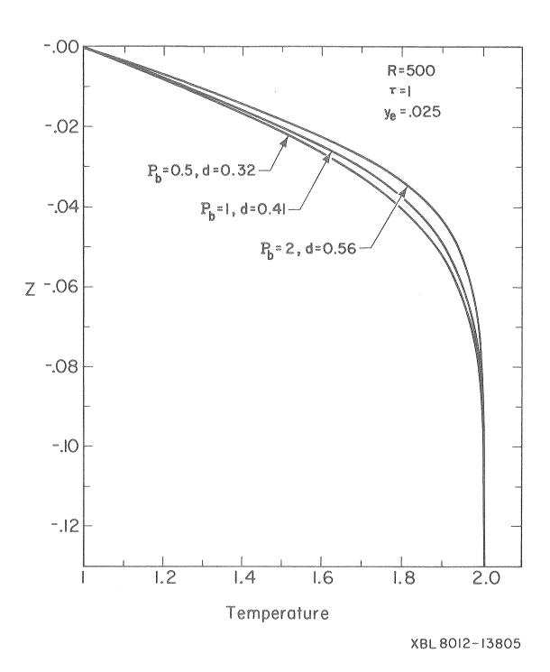
Fig. 7. Fluid temperatures in the fault for various values of  $P_{\rm b}$ .
