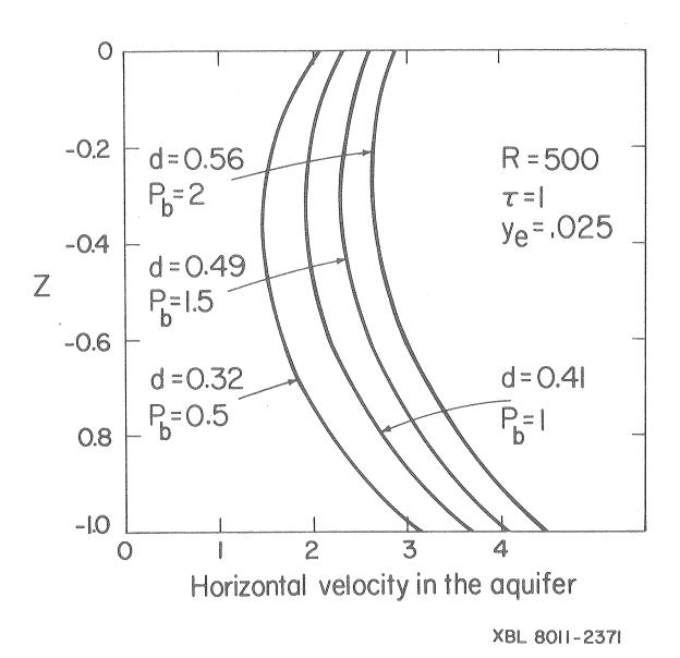
Fig. 6. Nondimensional horizontal liquid velocity in the aquifer along the depth of the reservoir for different values of  $P_b$ .
