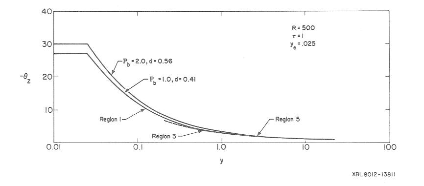
Fig. 10. Surface temperature gradients along the length of the aquifer for different values of  $P_{\rm b}$ .
