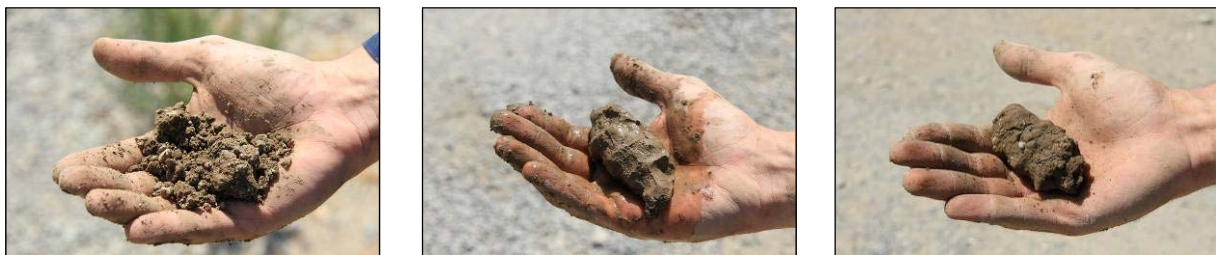
Figure 5.5: Squeeze test for assessing moisture content.
