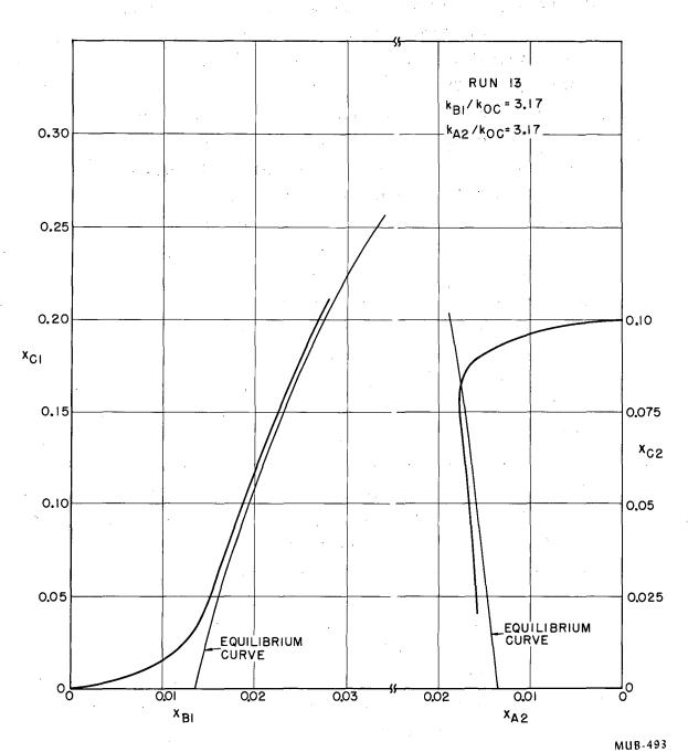
Fig. 6. Concentration profile for reverse extraction.
