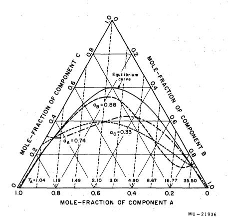
Fig. 1. Representative lines of constant-activity coefficients (γ<sub>A</sub>) and constant activity (a<sub>A</sub>, a<sub>B</sub>, a<sub>C</sub>).
