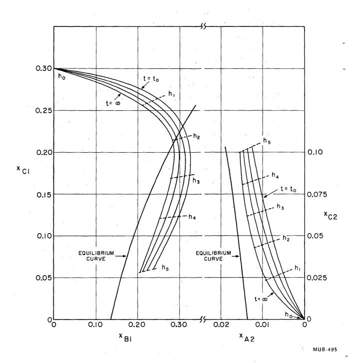
Fig. 9. Start-up behavior of an extraction column, with phase 1 continuous.
