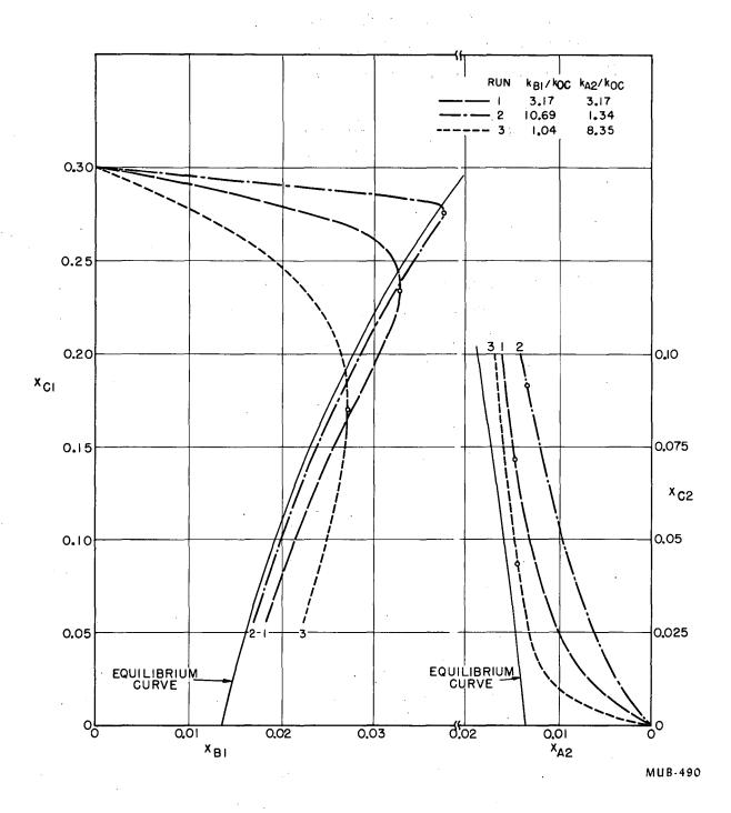
Fig. 3. Calculated concentration profiles showing the effect of the  $k_{\rm Bl}/k_{\rm Cl}$  ratio.
