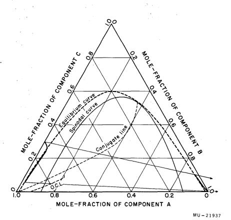
Fig. 2. Equilibrium diagram for idealized ternary system. Calculated concentration profiles shown for  $k_{C2}/k_{C1} = 1$ ,  $k_{B1}/k_{C1} = 1$ ,  $k_{A2}/k_{C1} = 1$  with points related by the operating conjugate line (O. C. L.).
