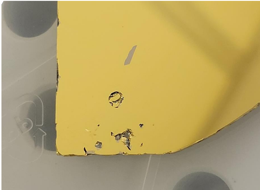
Figure 3.3.1. Corrosion of underlying silicon due to gold film discontinuities. Slight corrosion of the sample is also visible at the left edge. The bulk of the sample (both the gold film and the silicon wafer) is intact after two hours of HNA submersion.
