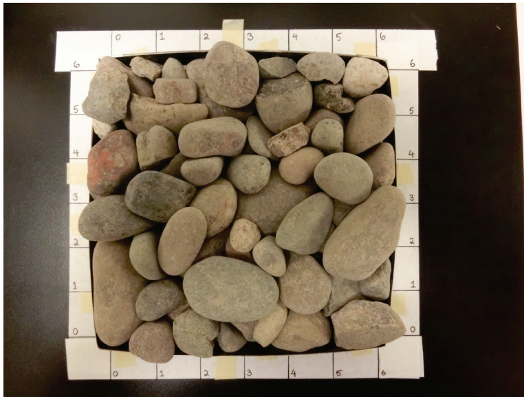
ESM Figure A-7. Images of aggregate A3 (1.5" multicolor ballast) showing (a) 4 m × 4 m target for E1918/E1918A and (b) 15 cm × 15 cm "box of rocks" for C1549. Code during testing was 3-3.
