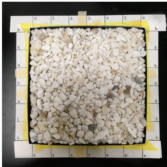
ESM Figure A-6. Images of aggregate A2 (3/8" white marble) showing (a) 4 m × 4 m target for E1918/E1918A and (b) 15 cm × 15 cm "box of rocks" for C1549. Code during testing was 3-2.
