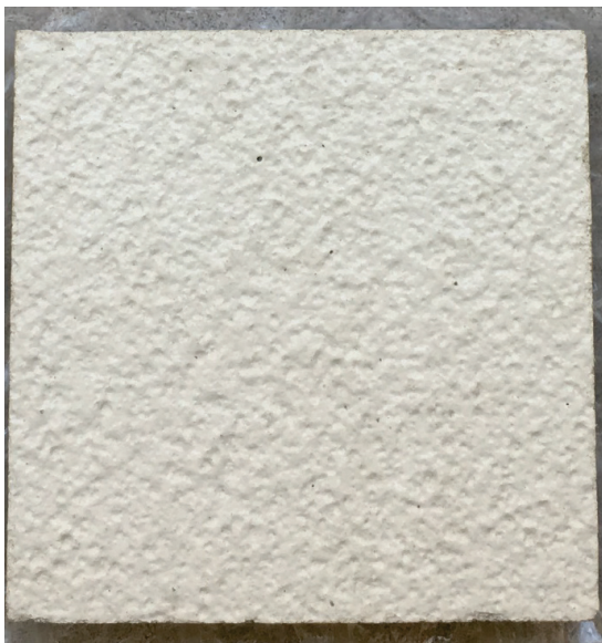
ESM Figure A-8. Images of tile T1 (white) showing (a) 4 m × 4 m target for E1918/E1918A and (b) 8 cm × 8 cm flat chip for C1549 and E903. Code during testing was 5-1.
