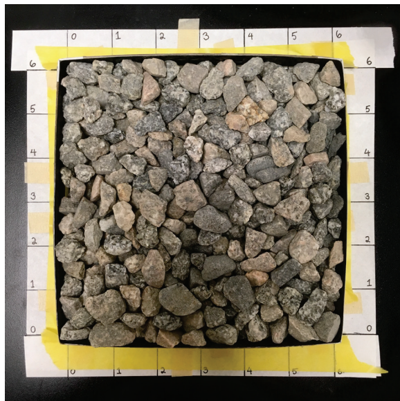
ESM Figure A-5. Images of aggregate A1 (5/8" gray granite) showing (a) 4 m × 4 m target for E1918/E1918A and (b) 15 cm × 15 cm "box of rocks" for C1549. Numbers in panel b mark inches. Code during testing was 3-1.
