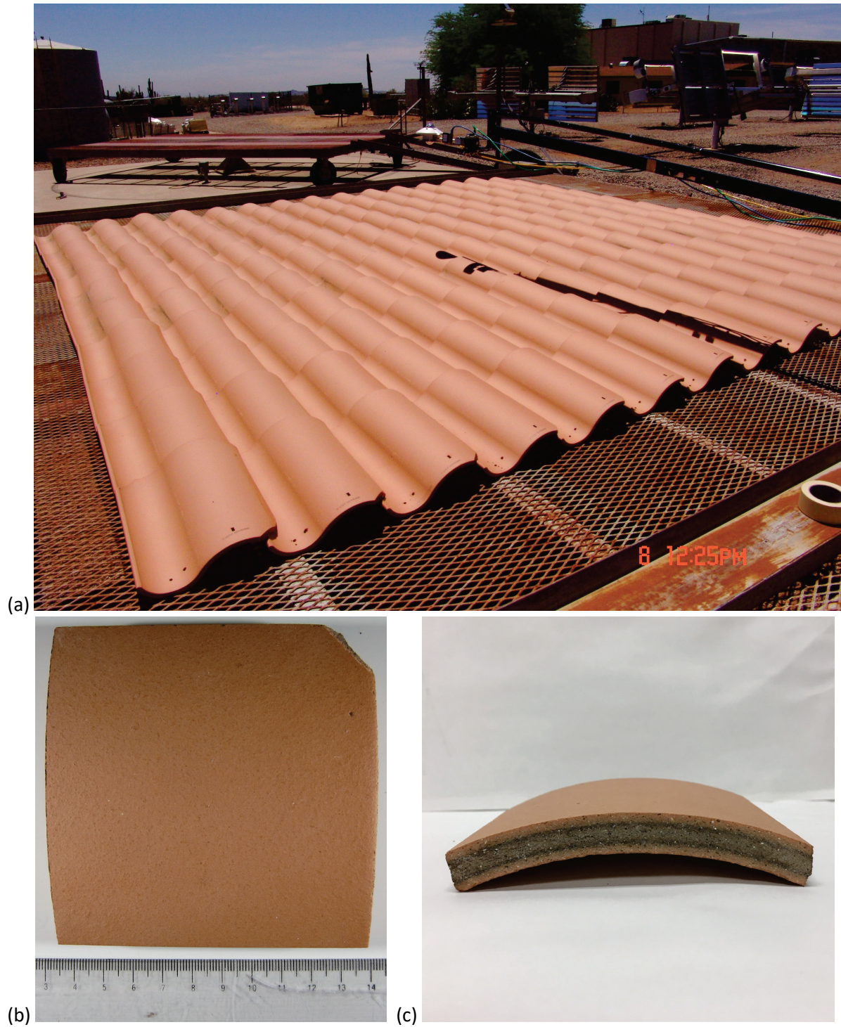
ESM Figure A-9. Images of tile T2 (orange) showing (a) 4 m × 4 m target for E1918/E1918A, (b) 10 cm × 10 cm curved chip for C1549 and E903, and (c) side view of curved specimen. Code during testing was 5-2.
