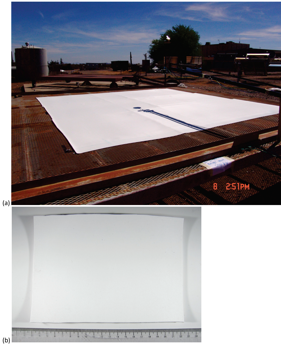
ESM Figure A-1. Images of membrane M1 (white) showing (a) 4 m × 4 m target for E1918/E1918A and (b) 15 cm × 20 cm coupon for C1549 and E903. Code during testing was 1-1.
