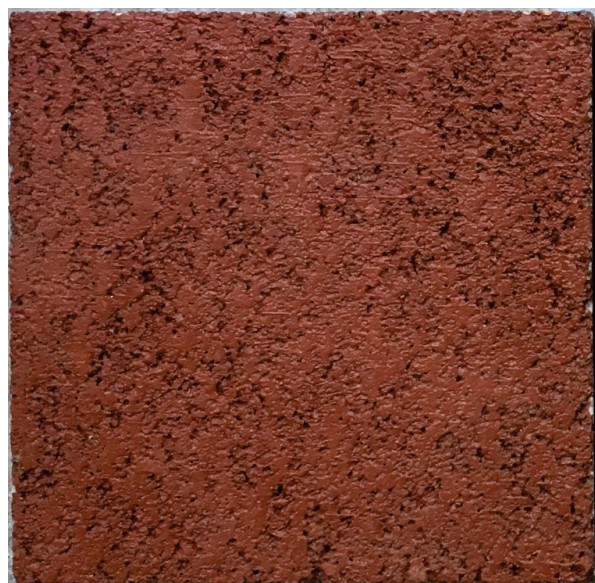
ESM Figure A-10. Images of tile T3 (red) showing (a) 4 m \times 4 m target for E1918/E1918A and (b) 8 cm \times 8 cm flat chip for C1549 and E903. Code during testing was 6-2.
