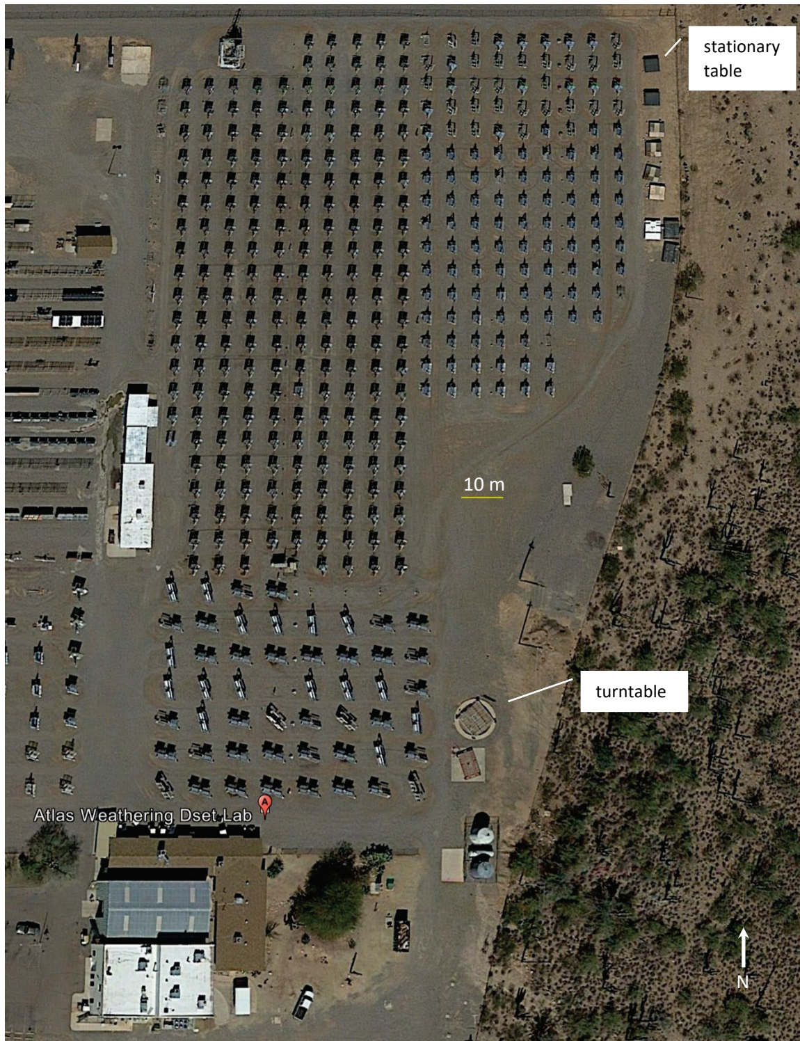
Figure 5. Atlas Weathering DSET Lab site image locating turntable used for E1918/E1918 measurement of membrane, shingle, and tile albedo, and stationary table used for E1918/E1918 measurement of aggregate albedo. Image source: Google Earth.
