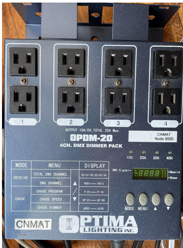
Figure 22. OPDM-20 DMX Control (fan plugged in here)
