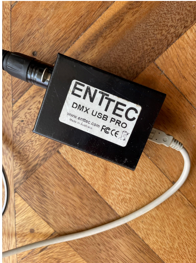
Figure 23. DMX to USB converter (connected to computer)
