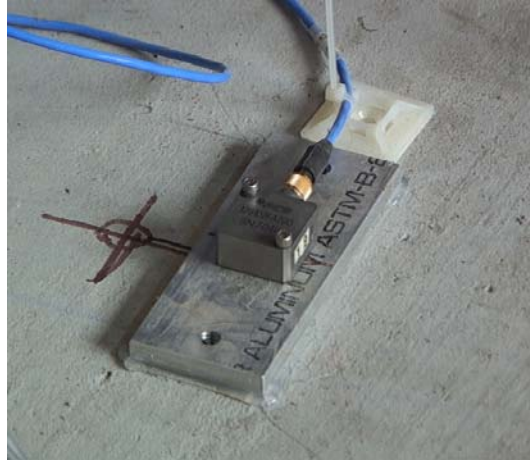
Figure 3-2 Sample Mounting of Accelerometer Mounting on Concrete Surface
