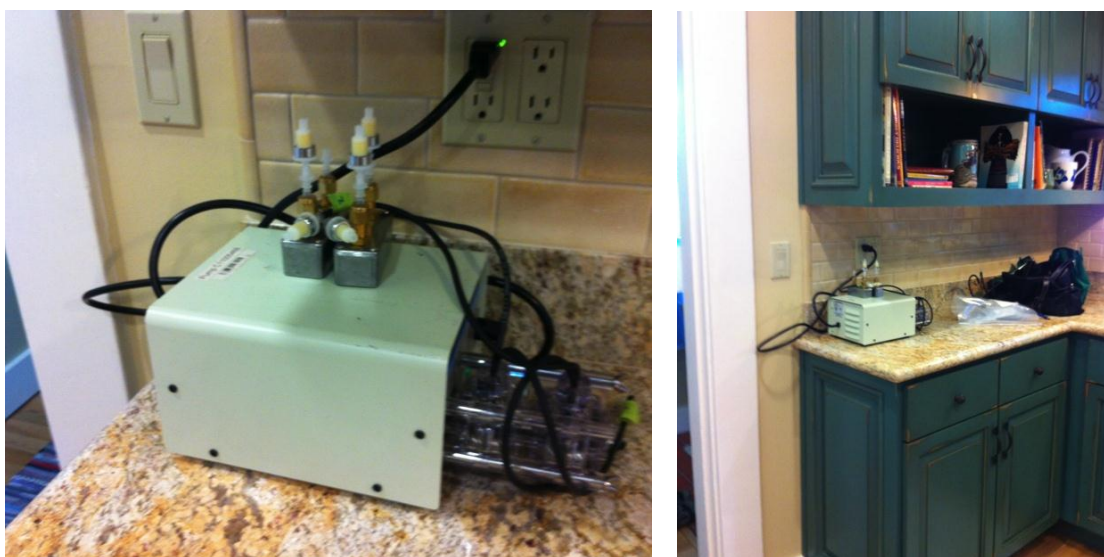
Figure 2. Placement of the three passive and two active samplers during the six-day passive sampling rate field experiment at site H5.
