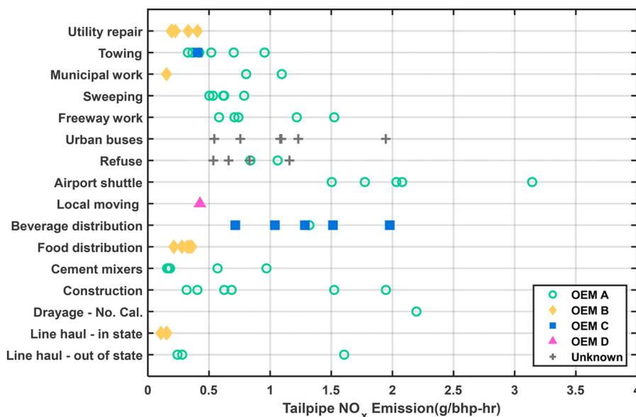
**Figure 1.** Brake-specific tailpipe NO<sub>x</sub> emissions of 72 HDDVs. Markers distinguish Original Equipment Manufacturers (OEM).
