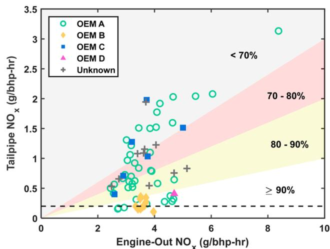
**Figure 3.** Engine-out and tailpipe  $\text{NO}_x$  emissions of 68 HDDVs. Points represent the average engine-out and tailpipe emissions of individual vehicles when both SCR inlet and outlet  $\text{NO}_x$  sensors were active. Different symbols represent vehicles with different engine makes, and shaded areas represent different  $\text{NO}_x$  conversion efficiency ranges. The dotted line represents the  $0.20 \text{ g/bhp-hr NO}_x$  standard.
