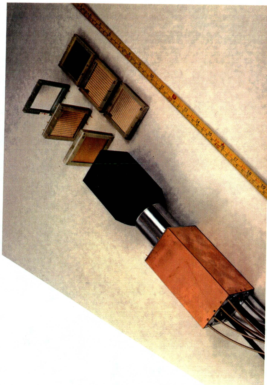
Figure II.11 Photograph of one of the Si-Si(Li)-Si(Li)-plastic telescopes used in the 80 and 100 MeV/u experiments. The alternating Au and Pd (dark lines) strips used for the position determination are visible on the front face of the 5 mm Si(Li) detectors.
