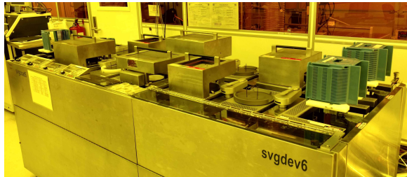
(a) A photoresist spin coater (svgcoat6) on the left right up against a photoresist developer (svgdev6) on the right. These machines are track systems that shuttle the wafer from one end to the other.
