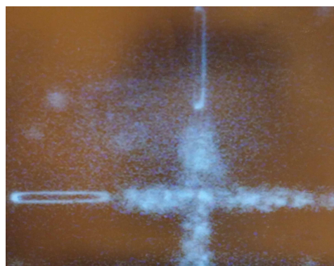
(d) An image from the CCD camera showing the two sets of alignment marks when the wafer are well aligned. The ground-plane slots are approximately 30\ \mu\text{m} in width; from this image, then, we can say that the alignment is good to approximately 10\ \mu\text{m} .
