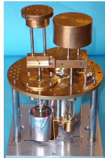
(b) Chase He10 fridge. The orientation here is upside down. (Image credit: Chase Research Cryogenics.)
