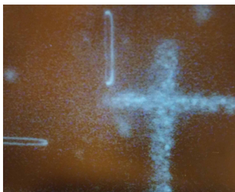
(c) An image from the CCD camera showing the two sets of alignment marks when the wafers are misaligned. The white chalk-like features are the back-illuminated slots in the ground plane of the device wafer. The thinner outlined streaks are the trench etches in the lenslet array.
