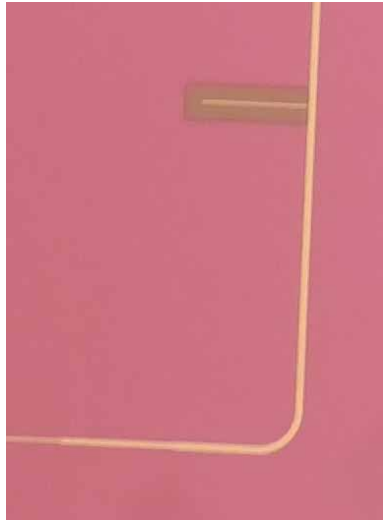
(a) A fabricated CPW 1-pole bandstop filter.
