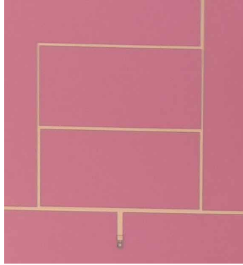
Figure 5.13: Fabricated double-ring hybrid tuned for a 150-GHz band. The orientation of this image is the same as that of the circuit diagram in Fig. 5.11(b). The sum port (port 4) is terminated with a lumped titanium resistor. Ports 2 and 3 feed the sinuous antenna differentially, and port 1 enters the summing network of the hierarchical phased arrays.
