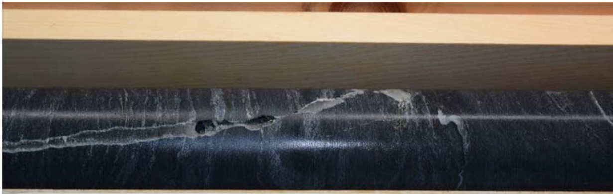
Figure 2.13. Open fracture encountered in kISMET-002 at ~91 ft (27.7 m). The fracture is lined with small quartz crystals, and is interpreted to be related to Tertiary-age mineralization.
