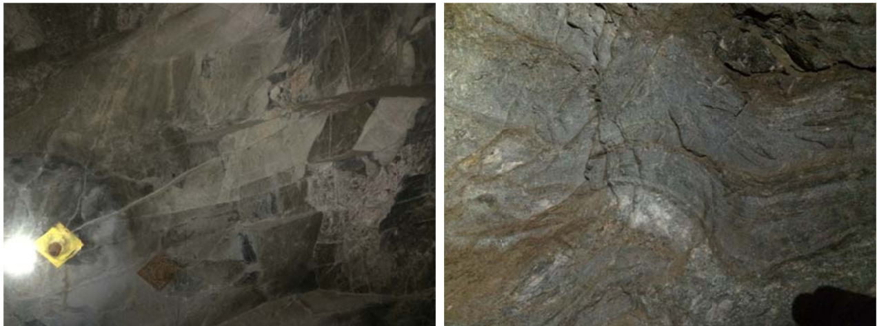
Figure 2.7. (a) Fractured and veined Yates amphibolite on 4100L; (b) Folded schist of the Poorman Formation on 4100L. Photos (both left- and right-hand images) are approximately 2 m across.
