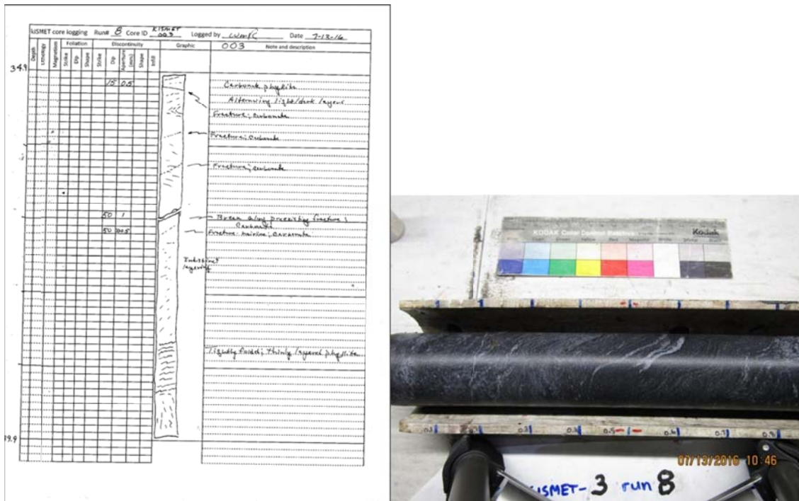
Figure 2.14. Examples of core descriptions (left-hand side image) and photographs from borehole kISMET-003, core run 8 (right-hand side image).
