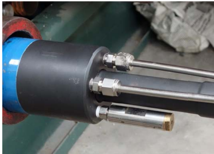
Figure 5.5. Top adapter on the straddle packer assembly shows the interval and the packer pressure lines and the normally-open relief valve. The parallel interval pressure line connected to the surface pressure transducer is hidden behind the stem connected to a wireline.
