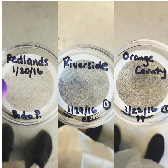
Figure 3-4: Photograph of three filter samples after particulate emission (RL1, WL1 and OL1). A color difference was observed for each filter sample.
