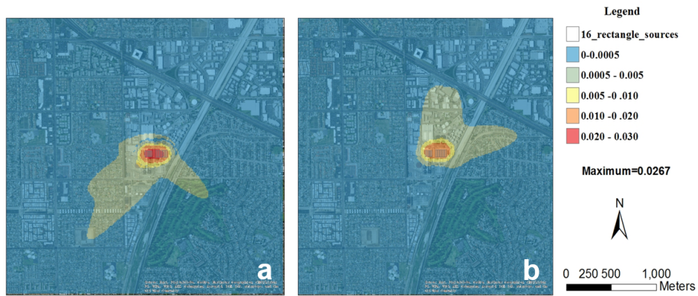
Figure 3-11: Modeled daily average concentrations of 16 uncovered rectangle sources. Runs were executed with meteorological data on a) February 15 th , 2012 and b) August 15 th , 2012.
