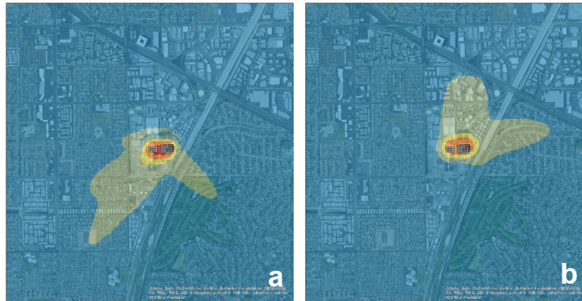
Figure 3-10: Modeled daily average concentrations of 84 semi-covered square sources. Legend remains consistent with figure 3-11. Runs were executed with meteorological data on a) February 15 th , 2012 and b) August 15 th , 2012.
