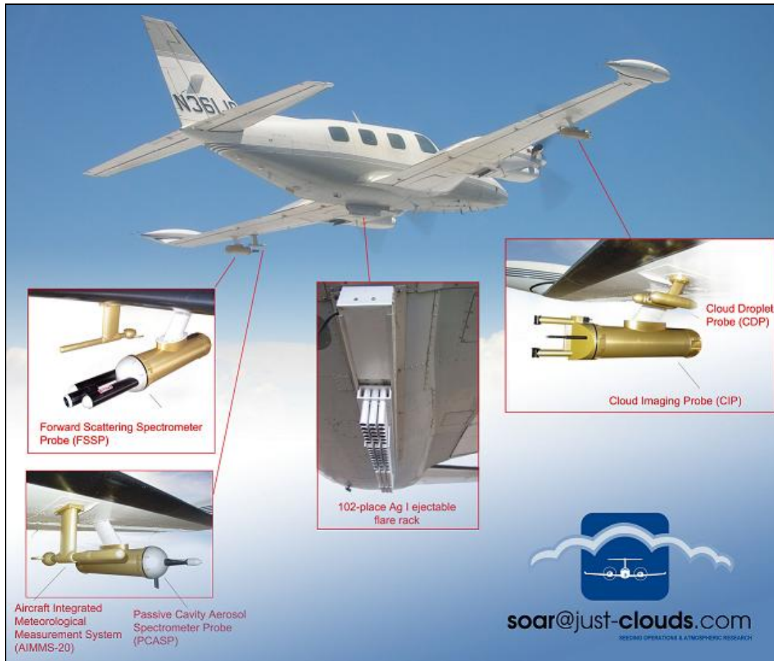
Figure 1. The SOAR Cheyenne II cloud physics aircraft
