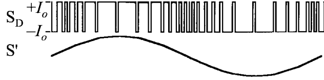
Figure 2.14: 2-level binary code used to generate the sine wave S' , the pulses in S_D represent the density of 1's and 0's in the bit stream [30].
