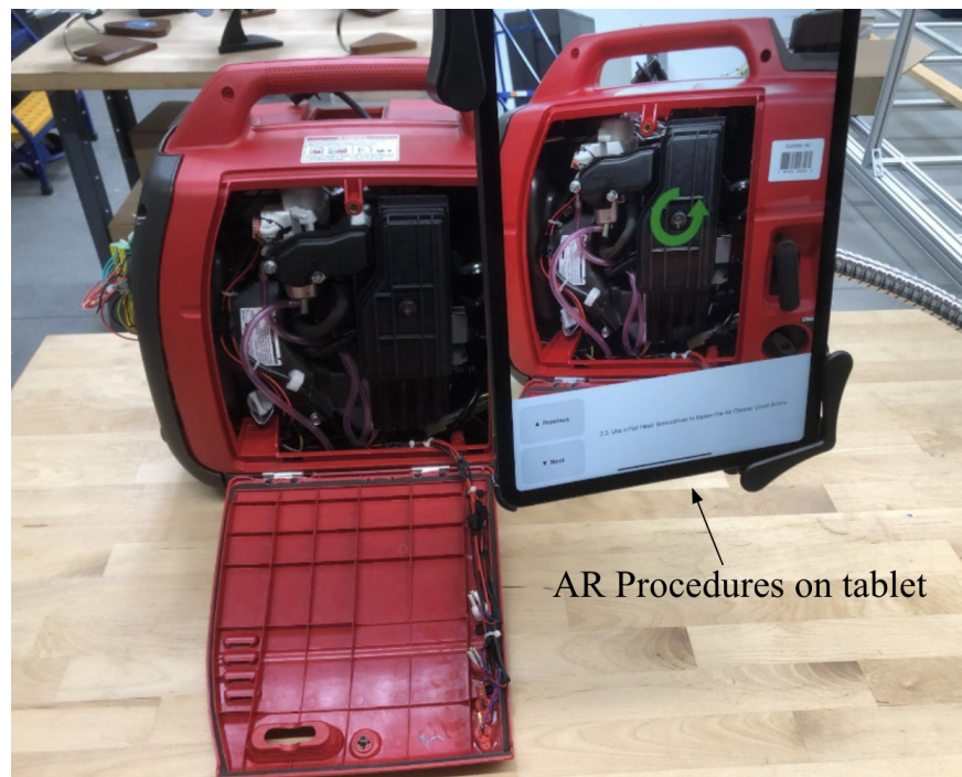
Figure 6.3: Augmented Reality Procedure system setup with tablet mount for hands free use.
