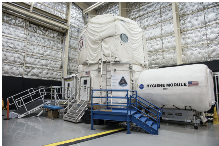
Figure 4.1: HERA, the Human Exploration Research Analog, is a three-story, closed habitat at NASA’s Johnson Space Center used to simulate long-duration human spaceflight missions (55).
