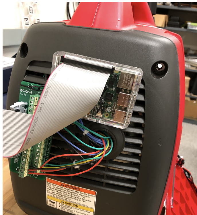
Figure 2.9: The Raspberry Pi microcomputer is hardwired to the embedded sensors and attached to the outside of the Honda generator.
