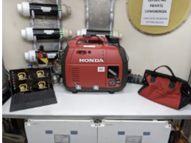
Figure 4.2: Experimental setup in HERA; the EPV is displayed on the tablet while the crewmember uses the tools on the right to perform the mechanical repair task on the generator.
