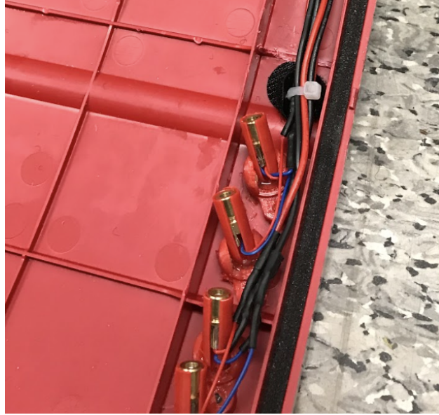
Figure 2.16: Lasers are placed into 3D printed housing and bolted to the front cover of the generator.
