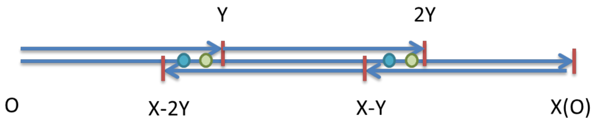
Figure 38. Diagram of candidate charging routes for BEV required at least two times fast charging.
