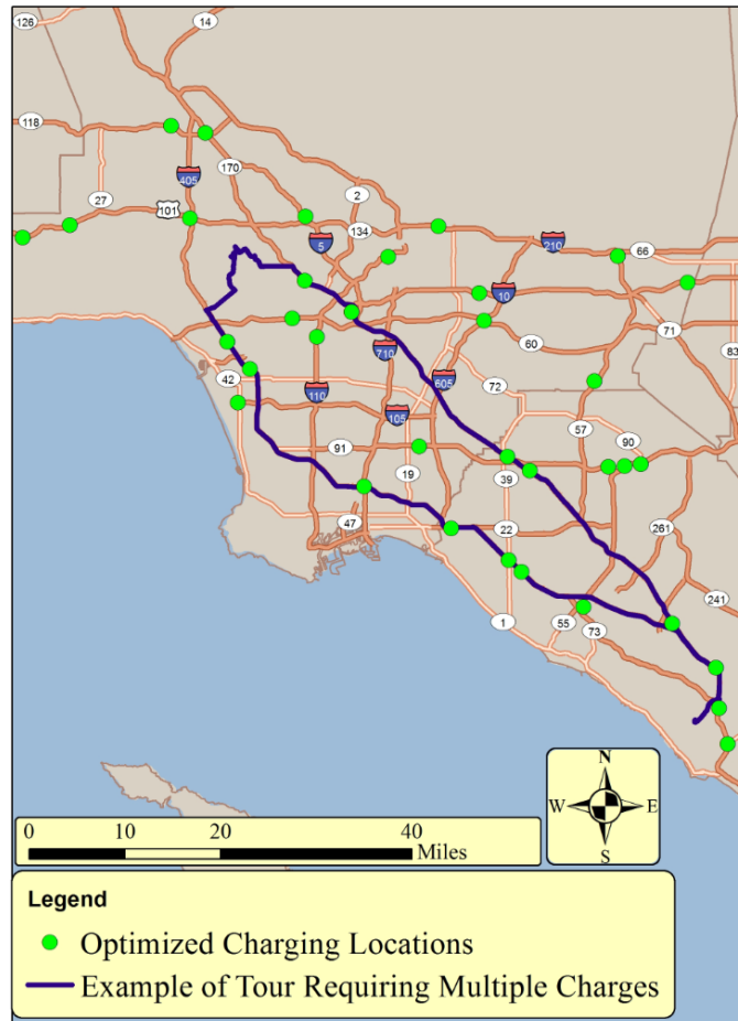
Figure 40. An example tour for a vehicle requiring multiple fast charging events.
