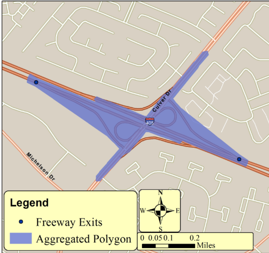
Figure 35. Aggregated polygon encompassing two freeway ramps and associated cross street.
