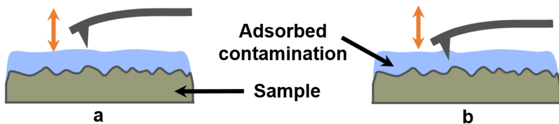
Figure 1.8: Challenges of NC-AFM imaging under ambient conditions: tip can be oscillating (a) above or (b) within the contamination layer on surface, leading to complications for atomic-resolution measurements.
