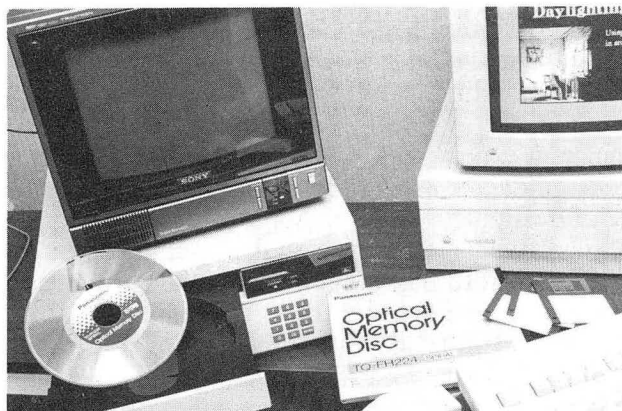
Fig. 6. The workstation today, with 8-inch analog optical discs, magnetic data discs, optical disc player, color video monitor and microcomputer. Future additions: CD-ROM data storage, digital optical storage, CD audio, and access to central network system. (XBB 894-3731)
