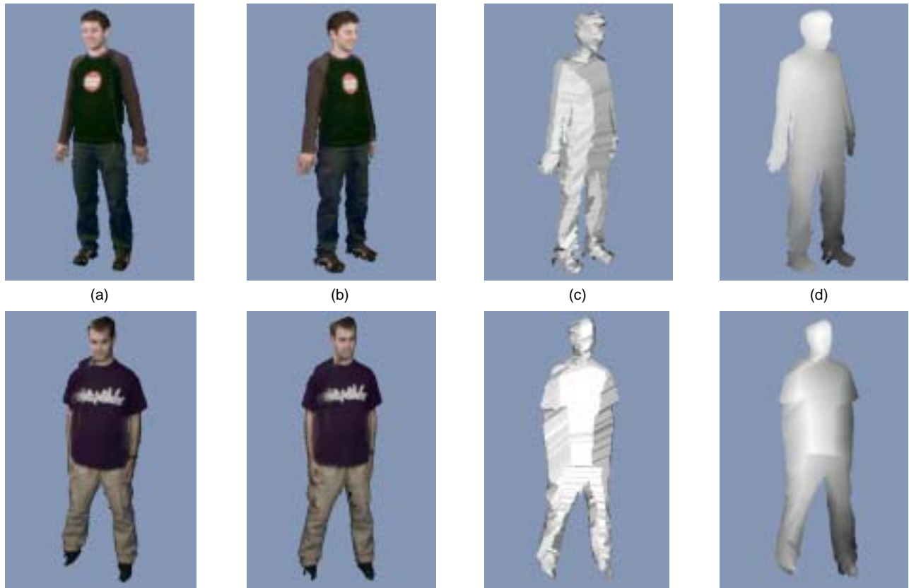
Figure 5: Images from 3D video sequences. (a) and (b) show surface splatted views from the 3D video. (c) reconstructed normals by flat-shading the view from (b) without colors. (d) is the corresponding depth map.
