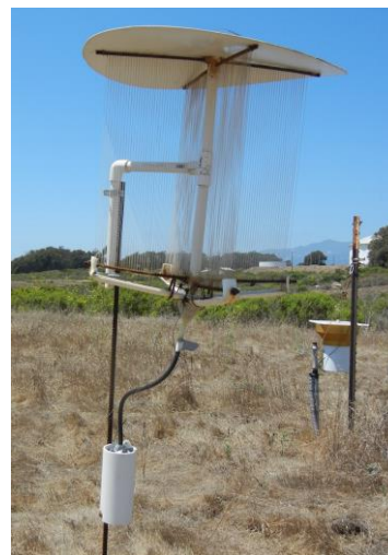
Photo of fog collector
